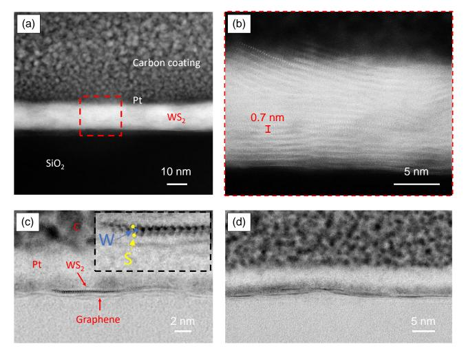
Figure 4. (a) Cross-sectional annular dark-field TEM image of  $WS_2$  electrodeposited for 5 min on patterned graphene electrodes. (b) High magnification image of the highlighted region in (a) showing the layer ordering of the 2D  $WS_2$  growing preferentially in the horizontal direction along the surface of the substrate. (c) and (d) Bright field TEM images of a film grown for 10 s showing regions of electrodeposited films composed of 1-2 layers over graphene.
