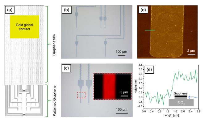
Figure 1 (a) Schematic diagram of the photolithography mask that was used in patterning the graphene electrodes. (b) Optical microscope image showing the graphene electrodes after fabrication. (c) Optical microscope image showing the graphene electrodes at higher magnification with a Raman map (inset) of the bare graphene. (d) AFM image of a graphene electrode after fabrication and a step height profile (e) taken at the edge of the electrode.
