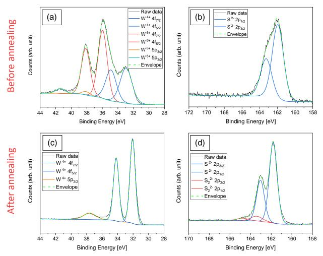
Figure 5 XPS measurements across the W (a) and S (b) binding energy range for the film before and after (c and d) annealing. The graphs show clear enhancement in the material crystallinity after annealing as evidenced by the reduction in the FWHM of the emission peaks and the increase in the intensity.
