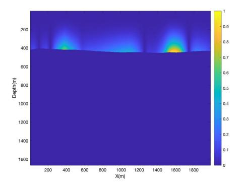
Figure 13. Prior fracture probability model obtained from the stress field.
