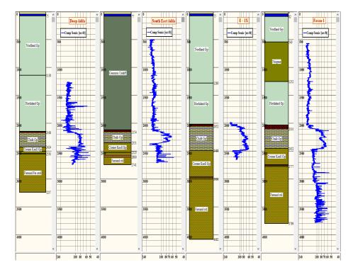
**Figure 2.** Overview of the sonic compressional logs (us/ft), acquired in the four wells. From left to right: Deep Adda, South East Adda, E-1X and Fasan-1. The depth reference is Rotary Table (RT, i.e. the rig floor).
