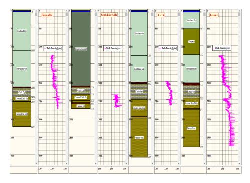
**Figure 3.** Overview of the density logs (g/cc), acquired in the four wells. From left to right: Deep Adda, South East Adda, E1X and Fasan-1. The depth reference is Rotary Table (RT, i.e. the rig floor).
