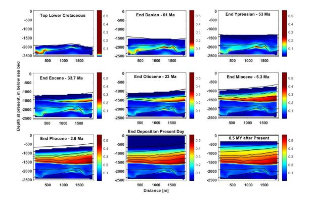
Figure 7. Evolution of the effective strain as result of the deposition of the Post-Chalk sediments.
