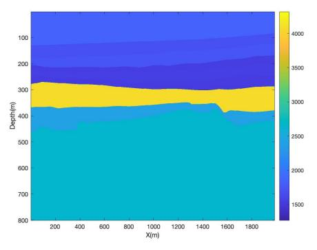
Figure 10. The center velocity model obtained by simple interpretation.
