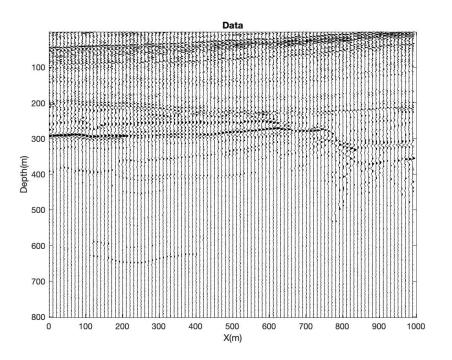
Figure 9. 2D observed seismic profile from the Tyra field.
