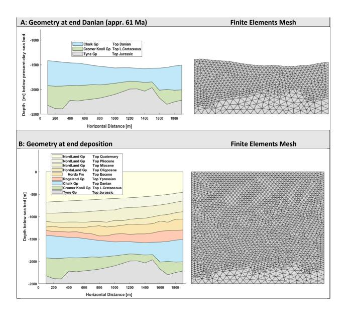
**Figure 5.** Model Geometry and the finite elements mesh in time. The depth is given meters [m] below sea bed at present. From top to bottom: a) Pre-existing domain (underburden) at time appr. 61 Ma (end Danian) before the onset of the overburden deposition; b) The final stage at present time after appr. 61 MY of deposition.
