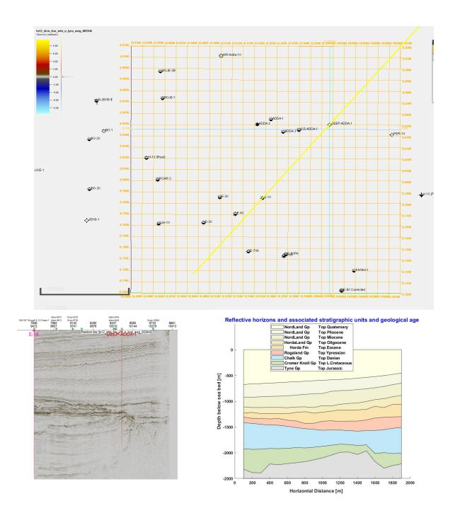
**Figure 4.** Sketch of the location of the considered seismic profile, the seismic data, and the main reflective horizons, derived from seismic interpretation and the corresponding stratigraphic units and geological age. The steep sections of the horizons representing the tops of the Jurassic and the Lower Cretaceous sections probably indicate the presence of faults.
