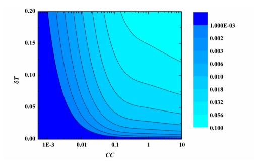
Figure 9. System error of  $\alpha_n$  caused by ignoring substrate temperature rise for various  $\delta T$
