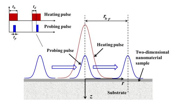
Figure 1. Schematic of the supported two-dimensional nanomaterial sample and the
