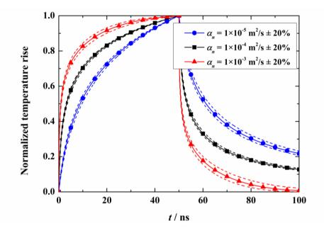
Figure 4. Normalized temperature rise curves of the supported sample for various  $\alpha_n$ (g/ $\lambda_n$ =3×10<sup>4</sup> m<sup>-1</sup>, heating pulse width  $t_h$  = 50 ns, temperature difference is assumed as 0.01 of
