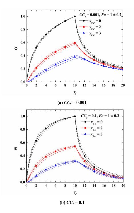
Figure 6. Normalized temperature variation curves at different positions with Fo changes ±20%
