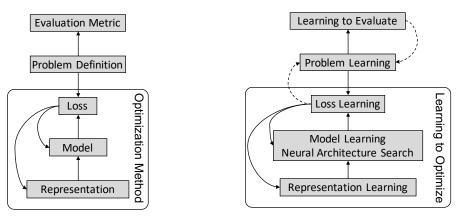
(a) A typical architecture of model AI systems. We first manually define a problem, and the problem decides the corresponding evaluation metric and loss function. Representations and a model are used to calculate the loss, which is minimized by some optimization algorithm so as to optimize the model and representations through back-propagation.
