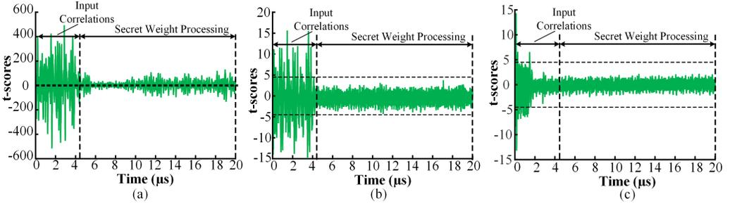
Fig. 15. First-order t-test results of the KSA-based design with PRNGs off (a), PRNGs on (b), and PRNGs on coupled with RSI shuffling of the node computations (c). (a) shows clear leakages throughout the execution, (b) only shows leakages during the input layer computations, and (c) shows a significantly lower leakage during the input layer computations as well due to the shuffle.
