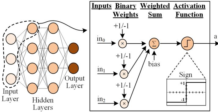
Fig. 2. A typical Binarized Neural Network where the neuron performs weighted summations of the input pixels with binarized weights, and the activation function is a sign function.
