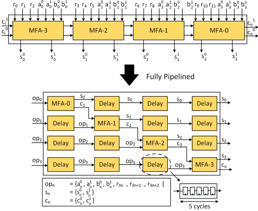
Fig. 7. Modular design of a masked 4-bit adder using Masked Full Adders (top) and its pipelined version (bottom). Pipelining ensures a throughput of 1 summation per cycle. where  $d^0, d^1, e^0, e^1, f^0,$  and  $f^1$  are the output shares from each Trichina Gate. From equations (3), (5), (6), and (7) we get
