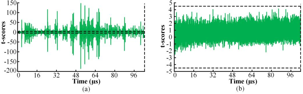
Fig. 16. First-order t-test results of the output layer computations in the KSA-based design with PRNGs off (a), PRNGs on (b). (a) shows clear leakages throughout the execution, whereas (b) shows that the t-scores stay confined to the threshold of  $\pm 4.5$ .
