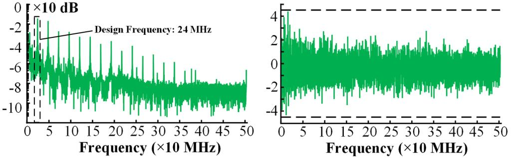
Fig. 17. Average frequency spectrum of masked Variant-III (left) and its TVLA result (right). The TVLA plot shows that there is no significant leakage in the frequency spectrum of the design when masked.
