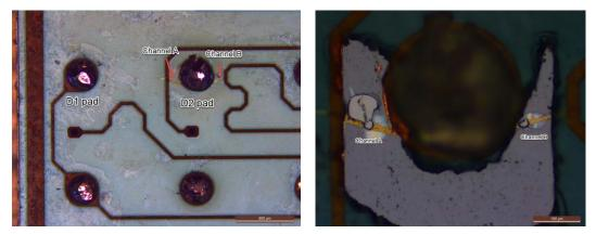
Figure 10 Left: Photomicrograph of faulty pad D2. Right: Photomicrograph after cutting off the conductive path Component analysis for Channel B.
