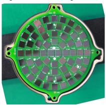
Figure 2 SiPM array of GRD
