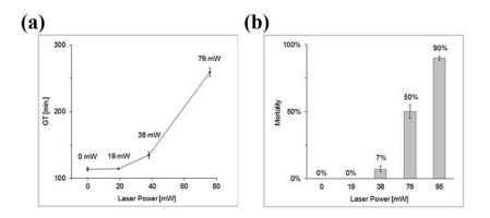
**Figure 9.** (a) Generation time (GT) of *S. cerevisiae* cells trapped for 15 min in optical tweezers with laser wavelength 1064 nm and trapping laser power in the range from 19 to 95 mW. The 0 mW point corresponds to the control unexposed cells. (b) Mortality (M) of optically trapped *S. cerevisiae* cells
