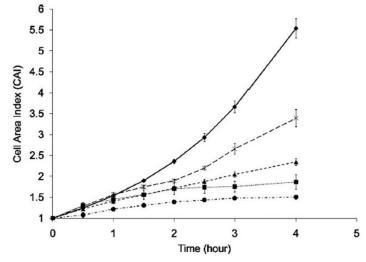
**Figure 7.** Effect of cw 1070 nm laser trapping on yeast growth (measured as Cell Area Index) for very long times (up to 4 h). Very low powers were employed (from top: control, 0.7 mW, 1.3 mW, 2 mW, and 2.6 mW). All powers produced a growth delay, the more significant the larger the power. A certain degree of adaptation can be observed for 0.7 mW and, perhaps, for 1.3 mW (note change in slope). (Reprinted with permission from Elsevier [80].).
