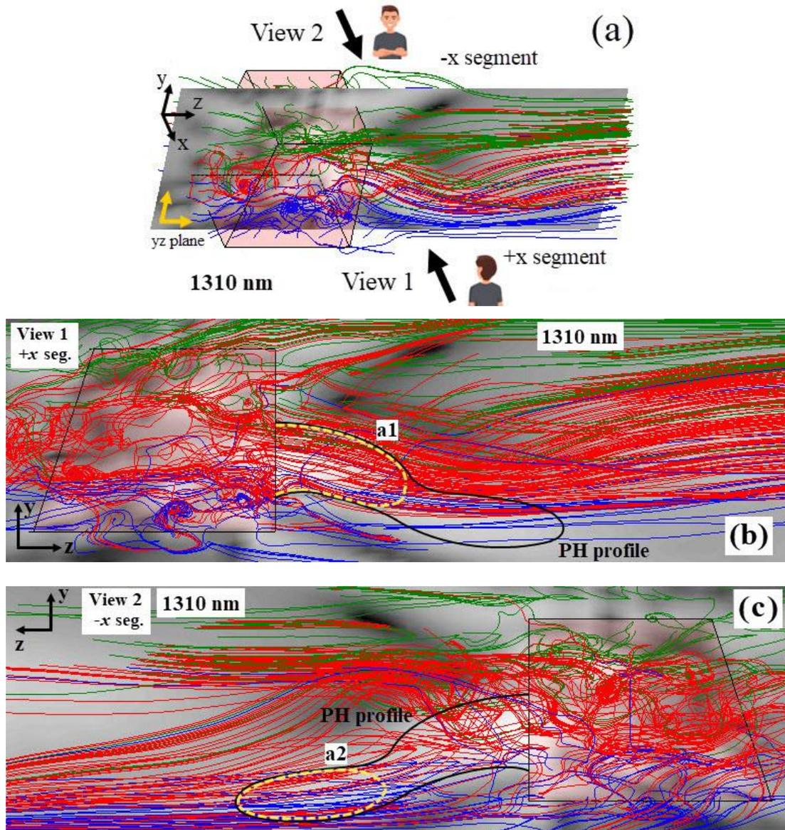
**Figure 4** (a) Diagram of view 1 and view 2 segments and 3D Poynting vector distributions for (b) view 1 +x segment and (c) view 2 -x segment of the model with the irradiation at the wavelength of 1310 nm. Orientations of the particle in (b) and (c) are reversed due to the change of frames of references for the observers in view 1 and view 2 as shown in (a).
