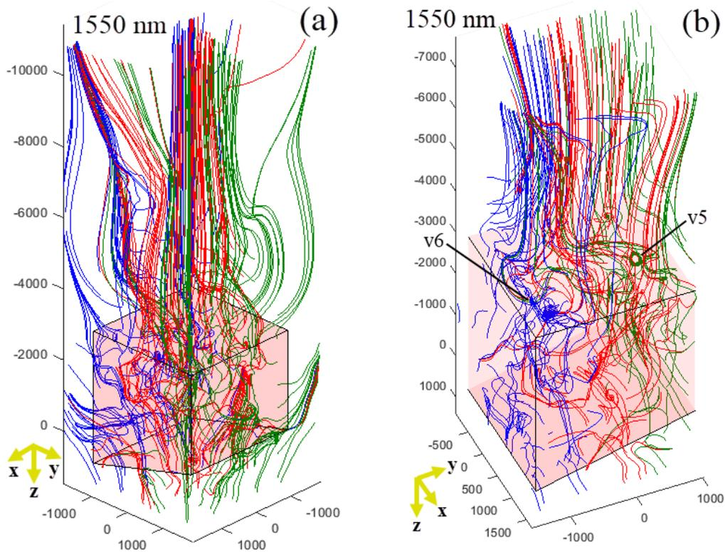
**Figure 5** Overview (a) and close-up view (b) of 3D Poynting vector distribution for the model of 1550 nm irradiation
