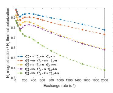
**Figure S6.** Maximum  $N_X$  achieved within 100 ms of CP transfer, as a function of the  $k_{HW}$  exchange rate. Different curves represent different sets of <sup>1</sup>H and <sup>15</sup>N relaxation parameters for protons and nitrogen. Notice the importance of water's relaxation: at fast exchange rates the labile proton acts as a mediator of polarization transfer, but the overall transfer efficiency is not dictated by their  $T_1/T_2$ , but rather by water's relaxation.
