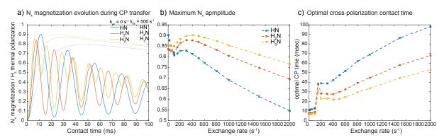
Figure S7. a) Amplitude of nitrogen buildup with three different spin systems in the absence and in the presence of fast chemical exchange. b) Maximum  $N_x$  amplitudes achievable for different chemical exchange rates and c) corresponding contact times needed for these amplitudes to be reached.
