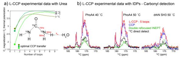
**Figure 10.** a) Experimental L-CCP results measured for urea's carbonyl <sup>13</sup>C in H<sub>2</sub>O at three different temperatures as a function of L-CCP looping. Starting point of buildups market with filled circles correspond to optimal CCP transfer at given temperature. b) Carbonyl spectra of unstructured proteins showing the superiority of CCP and L-CCP experiments comparing to INEPT or direct detect <sup>13</sup>C.
