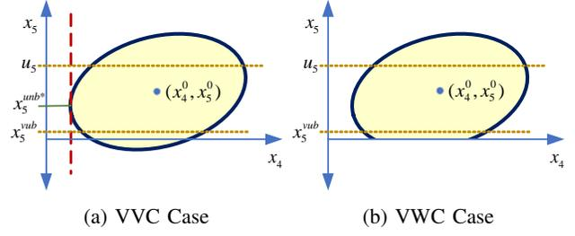
Fig. 2: Solution Space of the Distributed OPF
