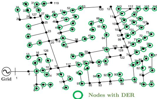
Fig. 3: IEEE 123 Bus Test System with 85 DERs
