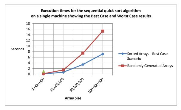
Figure 3 - Execution times in seconds when running a conventional version of the sequential quick sort algorithm on a single machine using integer arrays of different sizes, Table 1 in Appendix [A] presents the actual execution times for this graph.
