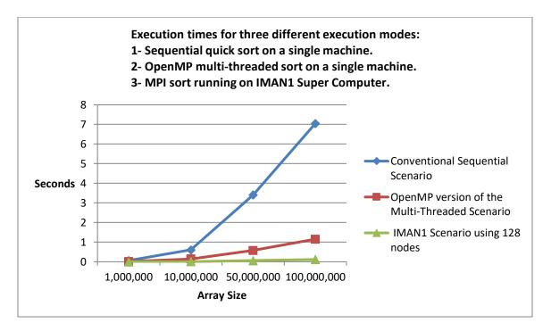
Figure 6 – Execution times for three different scenarios while sorting arrays of different sizes, the conventional sequential quick sort, OpenMP multi-threading experiments using (8) threads of execution and the IMAN1 super computer MPI experiments using (128) nodes.
