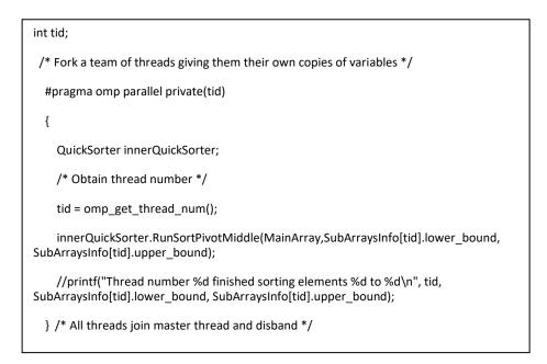
*Figure 5 – The simple C OpenMP code snippet that was used to enforce the usage of all the available processors on the test machine.*
