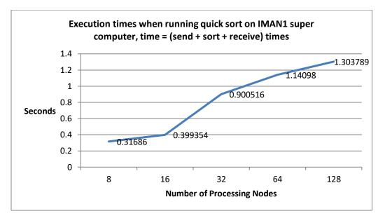
*Figure 6 – Execution time for the quick sort algorithm on IMAN1 super computer. The experiments were run using an initial array size of 5000000 elements while using different number of processors ranging from 8 to 128 nodes.*
