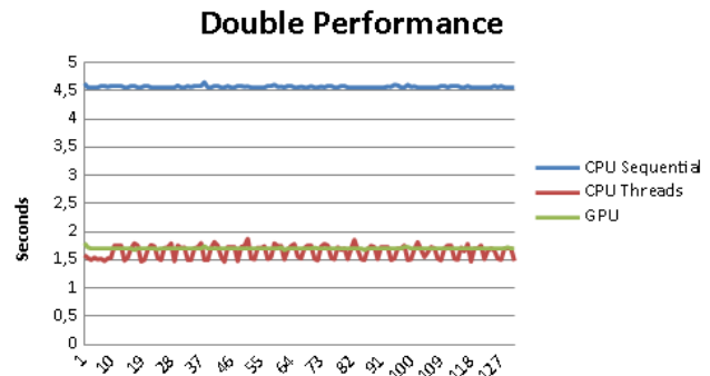
Fig. 6 Graphics with the performance of 2D image reconstructions using the 64-bit double data type.
