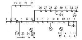
Fig. 1. IEEE 33-node network model from [24].
