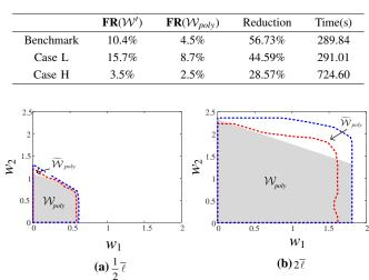
Fig. 7. The  $W_{poly}$  returned by Algorithm 2 under two current limits.
