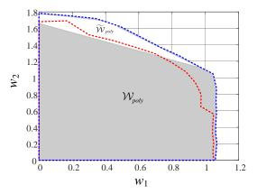
Fig. 4. The gray polytope  $W_{poly}$  is an approximation of W (red dash line). It is obtained by removing the output  $\tilde{W}_{poly}$  of Algorithm 2 (white polytope) from the output  $W'_{poly}$  of Algorithm 1 (the outside blue dash line).
