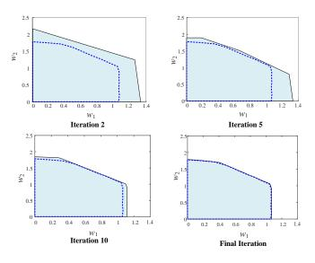
Fig. 3. The output of Algorithm 1 in different iterations (solid line) to approximate the SOCP-relaxed dispatchable region W' (dashed line).
