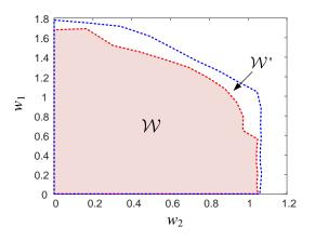
Fig. 2. The SOCP-relaxed region W' (outside) and the actual dispatchable region W obtained by checking sampled points in the  $(w_1, w_2)$  space.
