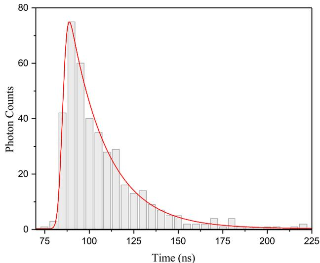
Figure 5: (Color online) Time decay curve of I<sub>2</sub> fluorescence for the  $E - B$  transition. The photon counting scan illustrating a histogram consisting of a range of time bins from the MCS. The red line is a convolution fit of a Gaussian with an exponential curve function to the data.
