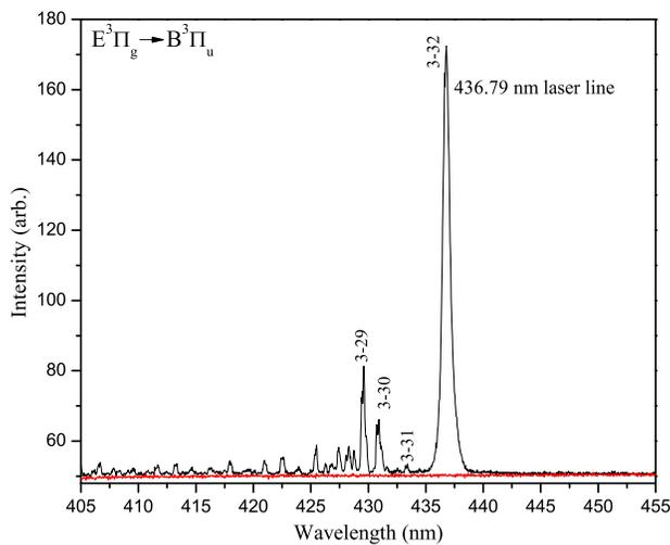
Figure 4: (Color online) The laser induced molecular fluorescence for the blue wing of the  $B^3\Pi_u^+(v' = 32) \leftarrow E^3\Pi_g^+(v = 3)$  emission is shown. Red line shows the background when laser 1 is blocked.
