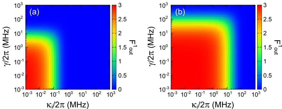
FIG. 6: Effect of intrinsic losses. (a) Dependence of the down-converted flux  $F_{\text{out}}^1$  on  $\gamma$  and  $\kappa_i$ , for  $(g, \omega_q, \omega_{\text{in}}) = 2\pi \times (0.3, 10.72, 8.9456)$  GHz and  $\kappa_e = 2\pi \times 255$  kHz. (b) The same plot as (a), for  $(g, \omega_q, \omega_{\text{in}}) = 2\pi \times (1.0, 9.735, 8.378)$  GHz and  $\kappa_e = 2\pi \times 35.4$  MHz.
