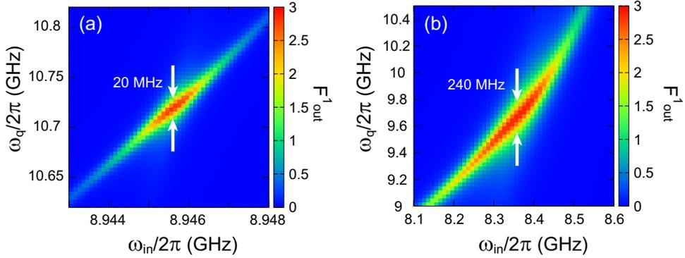
FIG. 5: Effect of qubit detuning. (a) Dependence of the down-converted flux  $F_{\text{out}}^1$  on  $\omega_q$  and  $\omega_{\text{in}}$ , for  $g = 2\pi \times 0.3$  GHz and  $\kappa_e = 2\pi \times 255$  kHz.  $\kappa_i = \gamma = 0$  is assumed. (b) The same plot as (a) for  $g = 2\pi \times 1.0$  GHz and  $\kappa_e = 2\pi \times 35.4$  MHz.
