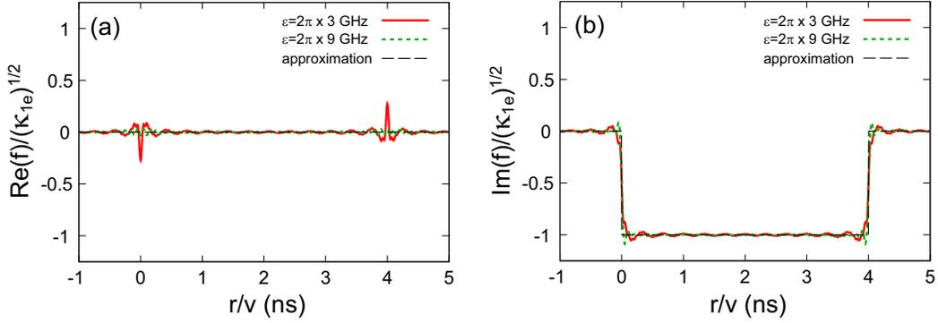
FIG. 8: Snapshots of  $f$  and  $f_{\text{app}}$  at  $t = 4$  ns: (a) real and (b) imaginary parts. Solid (dotted) lines represent  $f$  for  $\epsilon = 2\pi \times 3$  GHz (9 GHz), and thin dashed lines represent  $f_{\text{app}}$ . We assume a system-environment coupling of Eq. (28), and set the cutoff wavenumber at  $k_x = 2\pi \times 20$  GHz.
