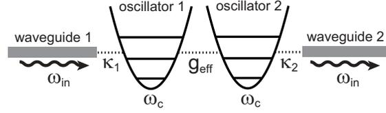
FIG. 9: Schematic of the coupled oscillators-waveguides system.
