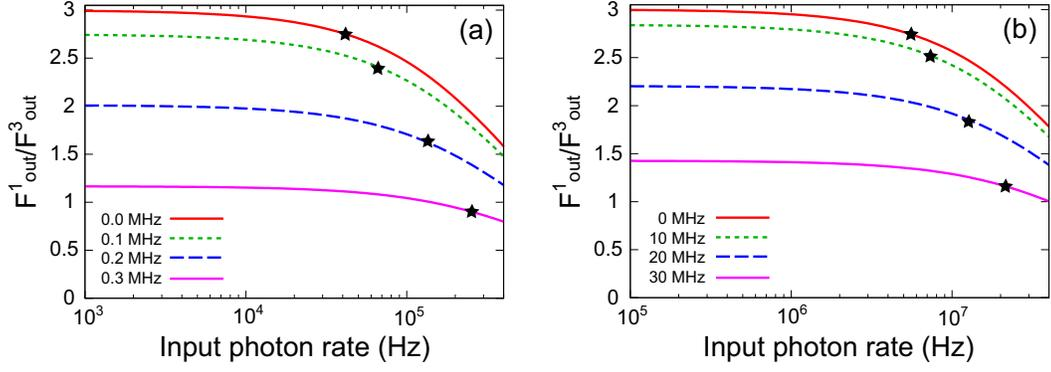
FIG. 7: Dependence of the down-conversion efficiency on the input photon rate. Detuning of the input photon frequency from the optimal one,  $(\omega_{\text{in}} - \omega_{\text{in}}^{\text{opt}})/2\pi$ , is indicated. Star symbols represent the onset of saturation [Eq. (30)]. (a) Results under the optimal condition in Fig. 4(a). (b) Results under the optimal condition in Fig. 4(b).
