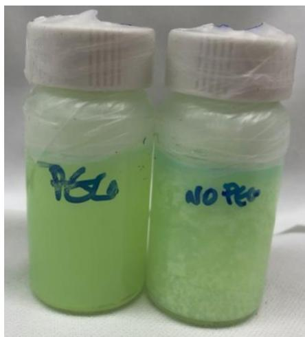
**Figure S4.** Photograph of UCNCs dispersed in water with and without the addition of MPEG-Silane. A precipitate rapidly forms (<1 hour) in the vial without MPEG-silane likely due to nanocapsule aggregation, and this aggregation is irreversible.
