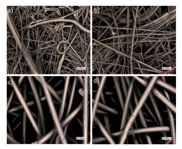
Figure 8: Laser microscope images of plasma treated / untreated FFP3 mask surface samples; a) untreated sample (area 1, 50x magnification), b) 15 h treated sample (area 1, 50x magnification), c) untreated sample (area 2, 50x magnification), d) 15 h treated sample (area 2, 50x magnification)
