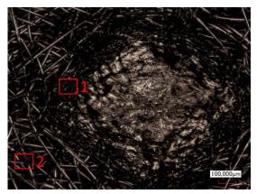
Figure 7: Laser microscope image of untreated FFP3 mask surface sample (10x magnification), locations marked in red are examples of the regions on the sample where the images in Figure 8 were taken (area 1: a) & b), area 2: c) & d))
