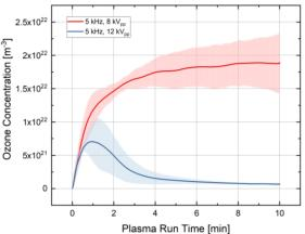
Figure 3: Ozone concentration in the SMD plasma chamber at 5 kHz and 8 kVpp / 12 kVpp
