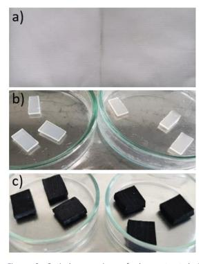
Figure 6: Optical comparison of plasma treated / untreated FFP3 mask samples and material samples; a) untreated (left) and 15 h plasma treated (right) FFP3 mask sample, b) untreated (left) and 15 h plasma treated (right) PP samples, c) untreated (left) and 15 h plasma treated (right) EVA samples
