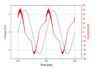
Figure 2: SMD discharge voltage and current at function settings of 5 kHz and 12  $kV_{pp}$
