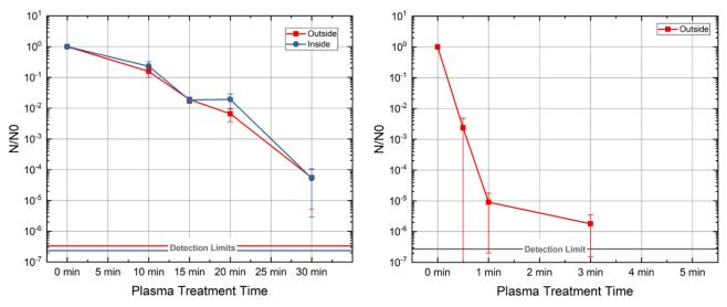
Figure 5: Results of the inactivation experiments in nitrogen mode ( $12 kV_{pp}$ , 5 kHz) with standard deviations; (left) inactivation of B. atrophaeus on FFP3 face mask samples from in- and outside of the mask, (right) inactivation of E. coli on FFP3 face mask samples from the outside of the mask
