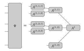
Figure 1. A diagram representing a ML-MCTDH approximation to a five-dimensional wavefunction. Each node of the tree corresponds to a coefficient tensor, and the lines connecting nodes represent the contraction over indices common to the two nodes.
