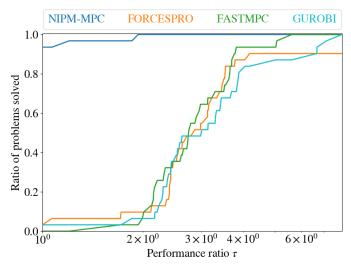
Fig. 2: Performance profile of the different IPM solvers for the 31 problems solved.
