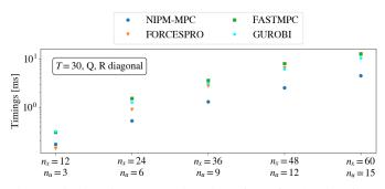
Fig. 4: Timings for Newton iterations for a fixed ratio of 4:1 between state to control variables. Q and R are diagonal matrices. NIPM-MPC is slower than FORCESPRO for  $n_x = 12$  but shows a flatter increase in computation times for a growing number of state variables.
