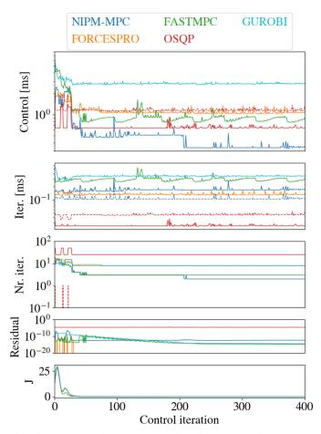
Fig. 5: Solver and control behavior for mass-spring system with  $n_x = 12$  and  $n_u = 3$ . Except for the cost J all graphs are in logarithmic scale for better readability.
