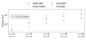
Fig. 6: Timings for Newton iterations for a fixed ratio of 4:1 between state to control variables. Q and R are dense matrices.
