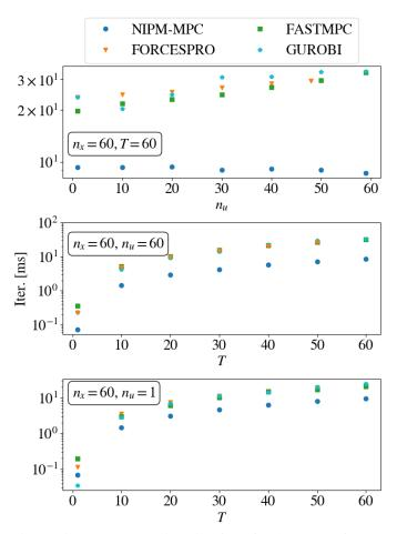
Fig. 3: Time per Newton iteration for a fixed number of states  $n_x$ . NIPM-MPC is consistently faster than FORCESPRO and FASTMPC and is outperformed by GUROBI only for  $n_x = 60$ ,  $n_u = 1$  and T = 1.
