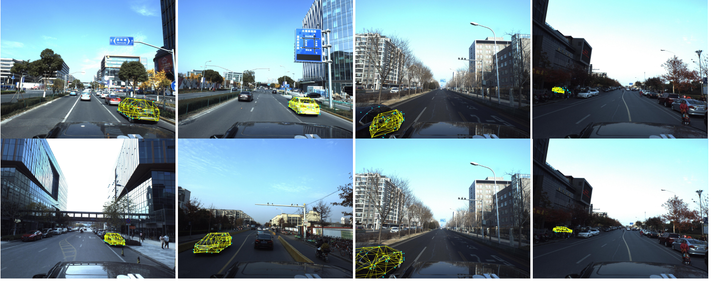
(b-1) Vehicle pose and shape estimation on ApolloScape [101]. Four examples where globally optimal estimates returned by GNC are certified by STRIDE.
