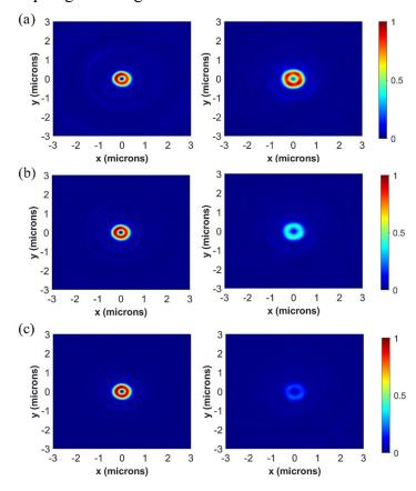
Fig.5 The intensity distributions of the focused vortex beams generated by Metalens 1 in different focal planes (left:  $z=12.3\mu m$ ; right:  $z=9.3\mu m$ ) when (a) ellipticity of the incident beam is 1/5, (b) ellipticity of the incident beam is 0, and (c) ellipticity of the incident beam is -1/5.
