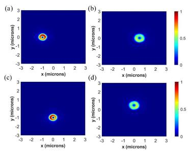
Fig.4 (a) and (b) are simulated intensity distributions of the focused vortex beams generated by Metalens 2 with different x-direction displacements in the same focal plane ( $z = 9.3\mu m$ ) for LCP and RCP incident beams, respectively. (c) and (d) are simulated intensity distributions of the focused vortex beams generated by Metalens 3 with different y-direction displacements in the same focal plane ( $z = 9.3\mu m$ ) for LCP and RCP incident beams, respectively.
