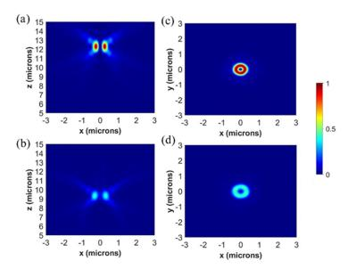
Fig.3 (a) and (b) are simulated electrical field intensity patterns in the x-z plane generated by Metalens1 under illumination of an LCP and RCP incident beam, respectively. (c) and (d) are simulated intensity distributions of the converged vortex beams in different focal planes (z =  $12.3\mu m$  or  $9.3\mu m$ ) for an LCP and RCP incident beam, respectively.
