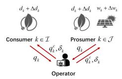
Fig. 1. Market structure of peer-to-peer energy sharing. Each consumer/ prosumer offers a bid  $q_k$  to the operator; the operator clears the market and returns the sharing profile  $q_k^c$  with the gap  $\delta_k$ . The users and operators are coordinated iteratively.
