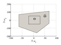
Fig. 4. Dispatchable region  $\bar{\Theta}$  (maximum set of  $\theta$  such that problem (8) has at least one feasible solution) and parameter range  $\Theta$  (we assume  $\theta \in \Theta$ ) of the 5-bus system.
