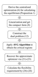
Fig. 2. A linear program (8) for computing the market equilibrium is derived based on Proposition 1 and linearization techniques. Then AVG algorithm is applied to calculate the flexibility requirement.
