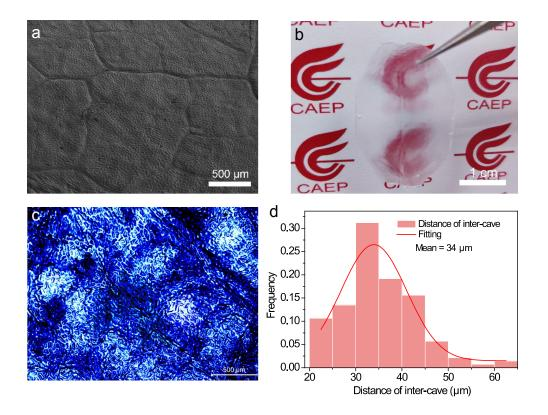
**Fig. S4.** a) SEM image of rose leaf. b) Photograph and c) top view optical morphology of rose leaf based bionic PDMS film. d) Statistical distribution of the distance of inter-cave in panel c, indicating the average interval gap of  $34\mu m$  and the coverage from 20  $\mu m$  to 65  $\mu m$ .
