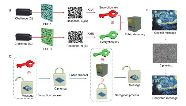
**Fig. 6.** Implementation protocol of bionic PUF based information encryption and transmission. a) Schematic of the generation of the encryption key and the decryption key. b) Mechanism of the encryption process and decryption process. c) A demo for encryption and transmission of painting *The Starry Night*.
