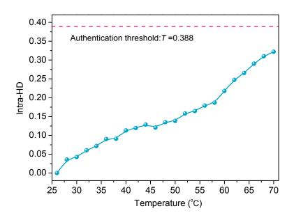
**Fig. S10.** Performance of the authentication protocol against thermal vibration. Intra-HDs ascend with increasing temperature while maintain below authentication threshold of 0.388, showing the reliability of PUF card within a certain temperature range.
