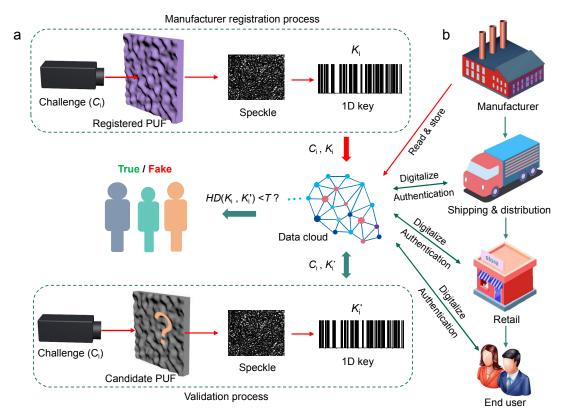
**Fig. 5.** An optical authentication system based on bionic PUFs. a) Schematic of registration and authentication processes. b) Schematic of the practical application of bionic PUF in the product verification covering the entire product supply chain.
