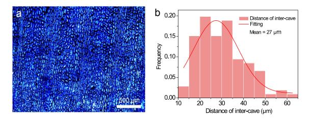
Fig. S5. a) Top-view optical morphology of ginkgo leaf based-bionic PDMS film. b) Statistical distribution of the distance of inter-cave in panel a, showing the average interval distance of 27  $\mu$ m and the coverage from 10  $\mu$ m to 65  $\mu$ m.
