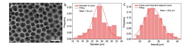
**Fig. S3.** a) Top view SEM image of rose petal based PVA film. b) Statistical distribution of diameter of the caves in panel a, showing the average diameter of 25  $\mu$ m and the distribution range from 14  $\mu$ m to 34  $\mu$ m. c) Statistical distribution of center point interval distance of the adjacent caves in panel a, demonstrating the average interval gap of 26.8  $\mu$ m and the coverage from 17  $\mu$ m to 42  $\mu$ m.
