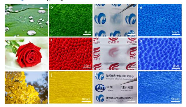
**Fig. 2**. Natural plants and bionic films. a) Photograph of a lotus leaf with rolling drops of water. b) A 45° titled view false-color SEM image of the lotus leaf. c) Photo image and d) surface morphology of the lotus leaf-based bionic PDMS film. e) Photograph of a red rose. f) False-color SEM image of the red rose petal. g) Photo image and h) 45° titled view false-color
