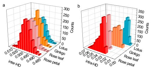
**Fig. 4.** Performances of bionic PUFs molded from different plant templates. a) Statistical distribution of the inter-HD for four kinds of bionic PUF molded from lotus, rose petal, rose leaf, and ginkgo, respectively. d) Statistical distribution of the intra-HD of these four kinds of bionic PUF outputs.
