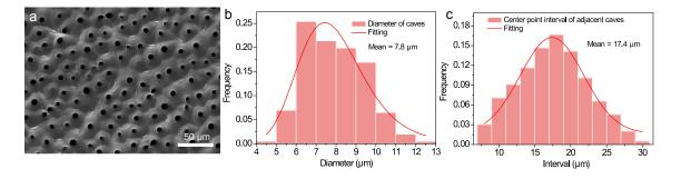
**Fig. S2.** a) Top view SEM image of lotus leaf based PDMS film. b) Statistical distribution of diameter of the caves in panel a, showing the average diameter of 7.8  $\mu$ m and the distribution range from 4  $\mu$ m to 13  $\mu$ m. c) Statistical distribution of interval distance of the adjacent caves in panel a, demonstrating the average interval gap of 17.4  $\mu$ m and the coverage from 9  $\mu$ m to 30  $\mu$ m.
