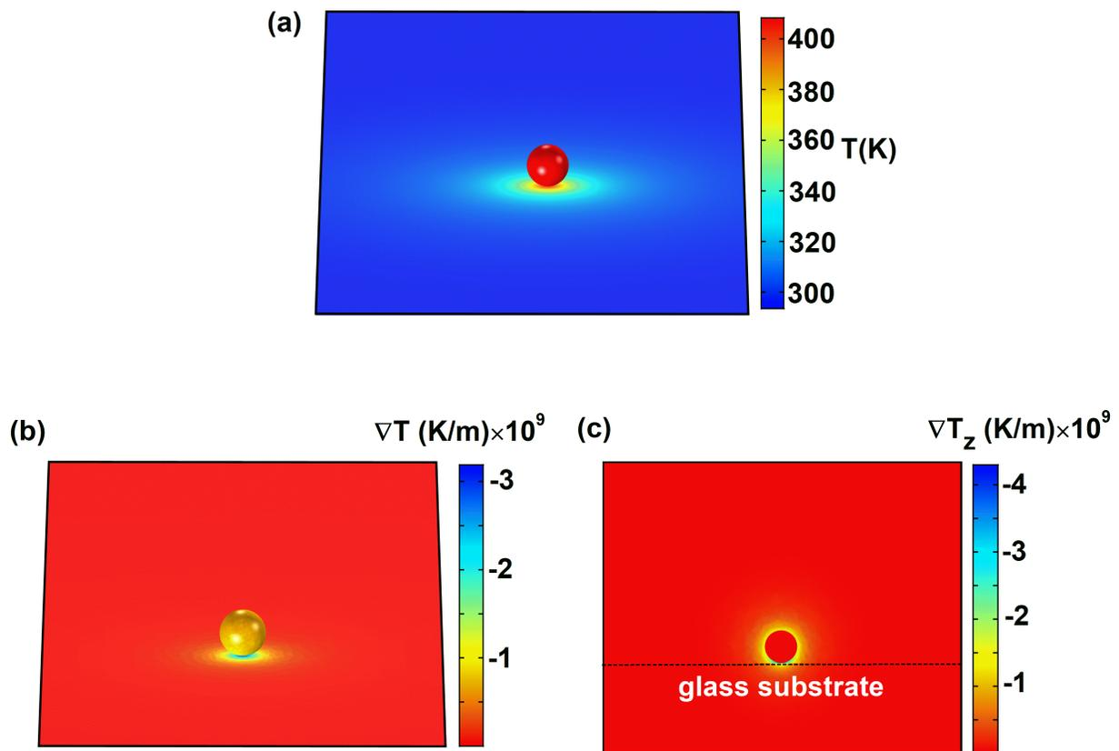
Figure S4: Calculated temperature and temperature gradient upon illumination of a single nanoparticle with a 532 nm laser at a power density of  $0.07 \text{ mW}/\mu\text{m}^2$ . (a) Temperature increment of the nanoparticle. (b) Calculated temperature gradient ( $\nabla T$ ) in the x-y plane and near the surface of the nanoparticle. (c) Calculated temperature gradient ( $\nabla T_z$ ) in the z plane.
