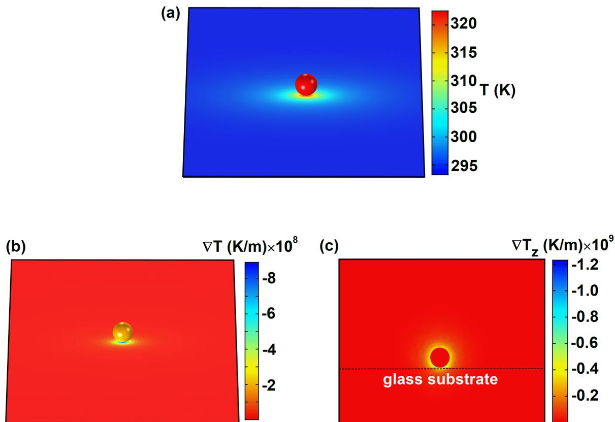
Figure S6: Calculated temperature and temperature gradient upon illumination of a single nanoparticle with a 633 nm wavelength laser at a power density of  $0.14 \text{ mW}/\mu\text{m}^2$ . (a) Temperature increment of the nanoparticle. (b) Calculated temperature gradient  $\nabla T$  in the x-y plane and near the surface of the nanoparticle. (c) Calculated temperature gradient  $\nabla T$  in the z plane.
