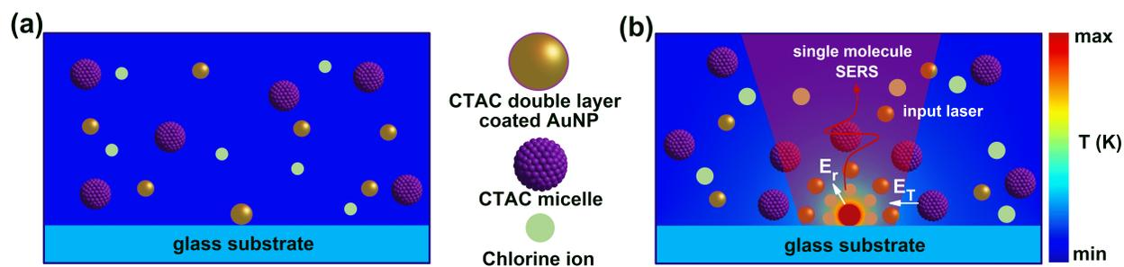
Figure S2: Detailed mechanism of the reversible trapping using single nanoparticle driven thermoplasmonic trap.
