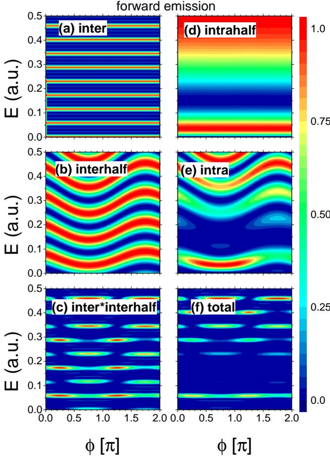
FIG. 13. Energy distribution in the forward direction as a function of the relative phase  $\phi$  for the  $\omega - 2\omega$  ionization within the SPA. (a) Intercycle factor, (b) interhalfcycle factor, (c) multiplication of (a) and (b), (d) intrahalfcycle factor, (e) intracycle factor [multiplication of distributions in (b) and (d)], and (f) the total momentum distribution [multiplication of (c) and (d)]. All distributions are normalized.
