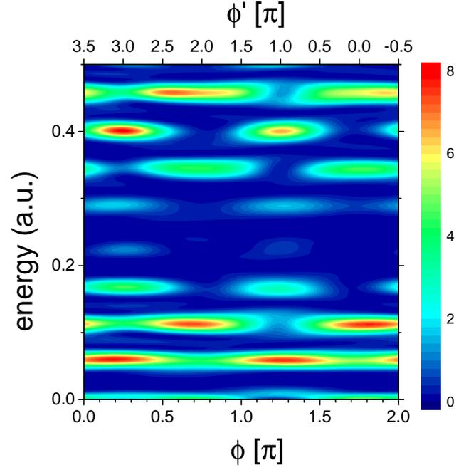
FIG. 14. Energy distribution in the forward direction as a function of the relative phase  $\phi$  for the  $\omega - 2\omega$  ionization within the SFA. In order to highlight the interference patterns we have multiplied the momentum distribution by  $\exp(15E)$
