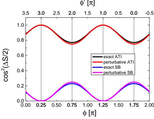
FIG. 12. SPA intracycle interference for ATI peaks and sidebands and their respective perturbative prediction both given by Eqs. (26) and (27) as a function of relative phases  $\phi$  (lower axis) and  $\phi'$  (upper axis) for  $\chi = 0.5$ . ATI maximizes at  $\phi = 0.25\pi$  and  $1.25\pi$  ( $\phi' = 3\pi$  and  $\pi$ ), whereas sidebands maximizes at  $\phi = 0.75\pi$  and  $1.75\pi$  ( $\phi' = 2\pi$  and  $0$ )
