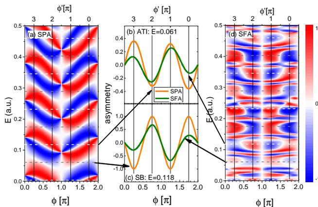
FIG. 15. Asymmetry parameter as a function of the energy  $E$  and relative phase  $\phi$  in (a) for the SPA and (d) for the SFA. The horizontal dash lines indicate the energy positions of ATIs (grey) and sidebands (white). In (b) the asymmetry parameter for the first ATI (at  $E = 0.061$ ) is plotted for the SPA and the SFA. In (d) the asymmetry parameter for the second sideband (at  $E = 0.118$ ) is plotted for the SPA and the SFA.
