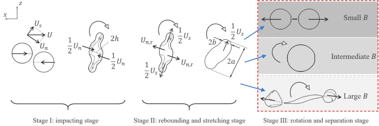
FIG. A1. Schematic of the model adopted in analyzing droplet reflexive and stretching separation for the collision between two non-spinning droplets.
