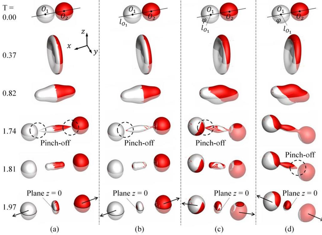
FIG. 4. Evolution of droplet deformation upon a head-on collision of (a) two non-spinning droplets and of a spinning droplet  $O_1$  and a non-spinning droplet  $O_2$  with varying azimuthal angle of droplet  $O_1$  (b)  $\varphi = 0$ , (c)  $\varphi = \pi/4$ , and (d)  $\varphi = \pi/2$ , at  $We = 61.4$ ,  $Oh = 0.028$ , and  $\omega_0 = 3$ .
