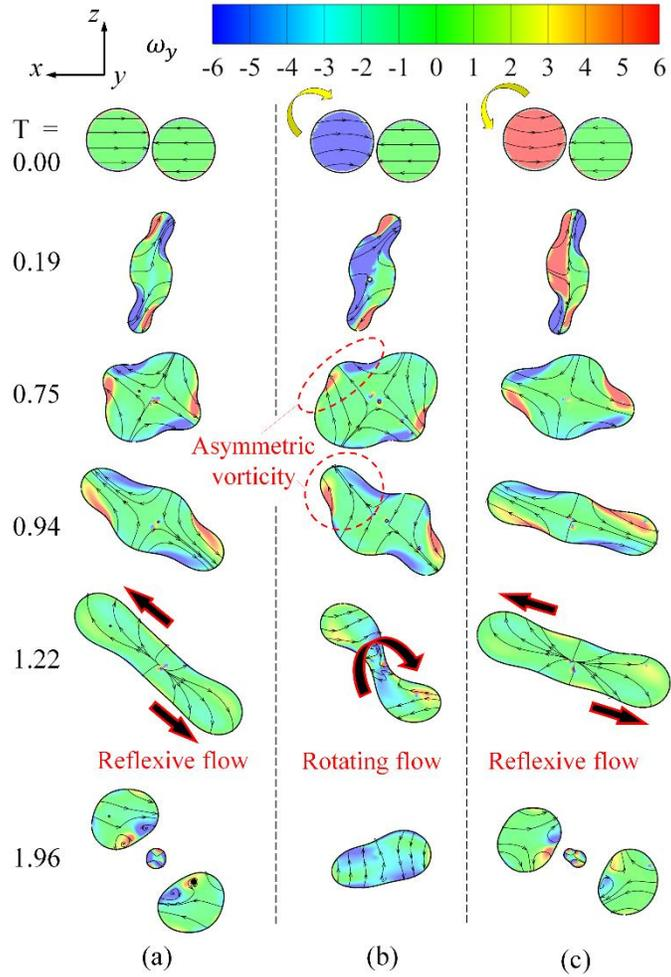
FIG. 11. Contour of the vorticity field and streamlines for droplet reflexive separation that shown in Fig. 10 for the case of (a) two non-spinning droplets and the cases of one spinning droplet with (b)  $\omega_0 \hat{y} = -3$  and (c)  $\omega_0 \hat{y} = 3$ .
