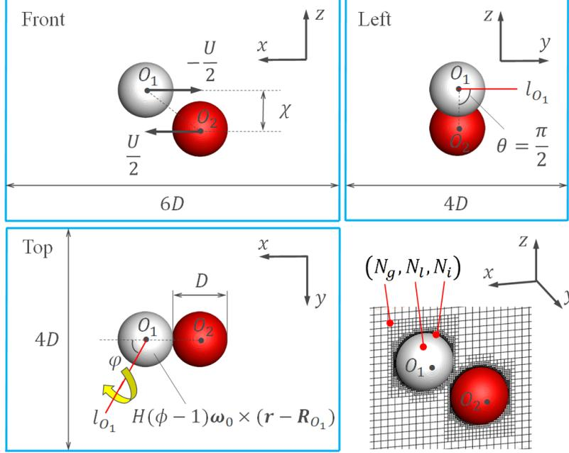
FIG. 3. Three-dimensional computational setup for an off-center collision between a spinning droplet  $O_1$  and a non-spinning droplet  $O_2$ .
