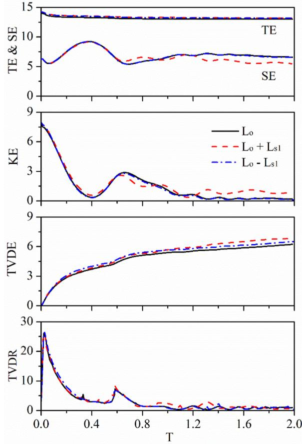
FIG. 10. Energy budget of the cases for the nearly head-on collision at  $We = 61.4$  and  $B = 0.15$  that are extracted from Fig. 9, in which the total energy (TE), the surface energy (SE), the kinetic energy (KE), the total viscous dissipation energy (TVDE), and the total viscous dissipation rate (TVDR) that are all nondimensional.
