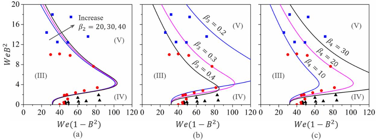
FIG. A3. Comparison of the predicted boundaries with different proportionality factors: (a)  $\beta_2$ , (b)  $\beta_3$ , and (c)  $\beta_4$ .
