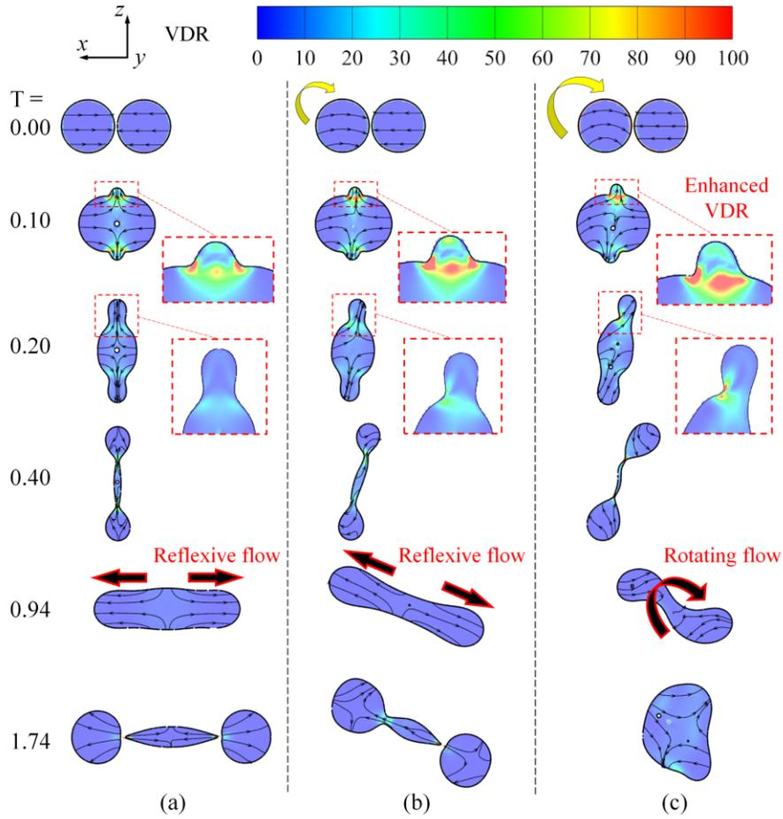
FIG. 6. Contour of the viscous dissipation rate (VDR) and streamlines for the three cases of reflexive separation at  $B = 0.0$  that shown in Fig. 5(a-c) with (a)  $\omega_0 = 0$ , (b)  $\omega_0 = 3$ , and (c)  $\omega_0 = 6$ .
