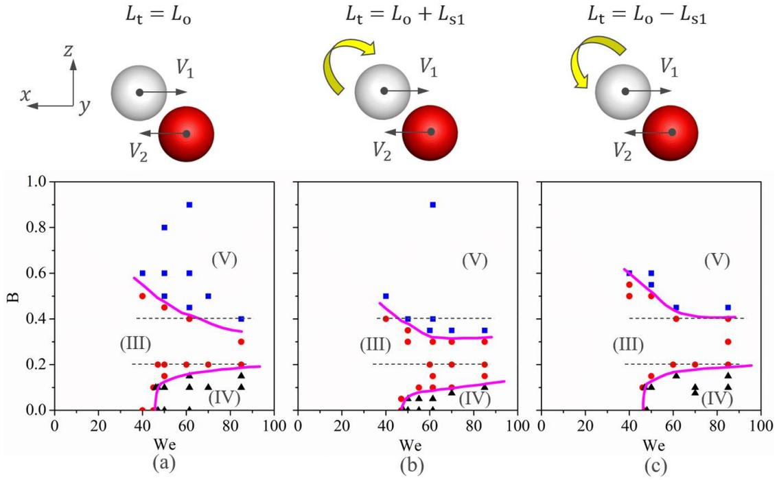
FIG. 9. Influence of chirality of droplet spin on the transition of coalescence-separation boundary at  $Oh = 0.028$  for the case of (a) two non-spinning droplets and the cases of one spinning droplet with (b)  $\omega_0 \hat{y} = -3$  and (c)  $\omega_0 \hat{y} = 3$ .
