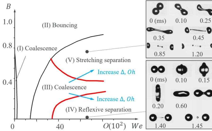
FIG. 1. Schematic of droplet collision regimes in a  $We - B$  parameter space and experimental images for reflexive and stretching separation[4] for collision of identical droplets in atmosphere.
