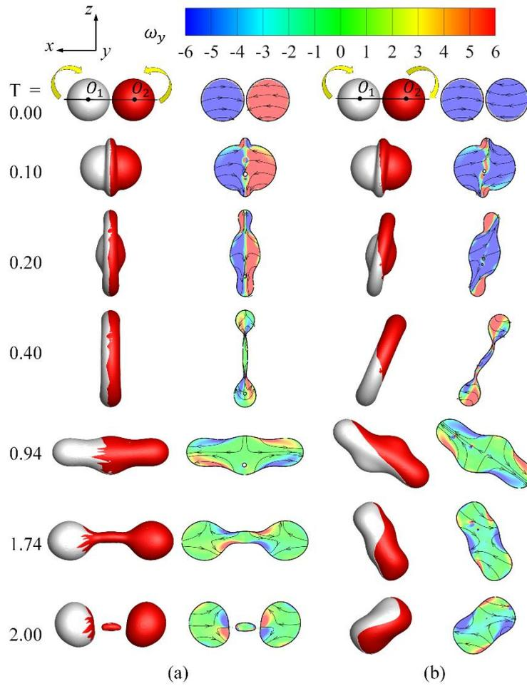
FIG. 12. Droplet deformation and vorticity contour for a head-on collision between two spinning droplets at  $We = 61.4$ ,  $Oh = 0.028$  and  $\omega_0 = 3$ . The spin motions have the (a) opposite direction and (b) the same direction.
