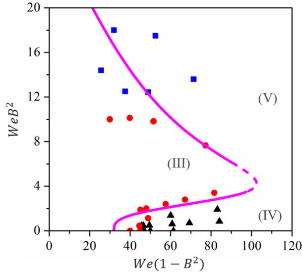
FIG. A2. Predicted boundary for the reflexive and stretching separation of two non-spinning droplets in the parameter space  $We(1 - B^2) \sim WeB^2$ . The dashed curve indicates the occurrence of droplet coalescence, which cannot be predicted by the present model.
