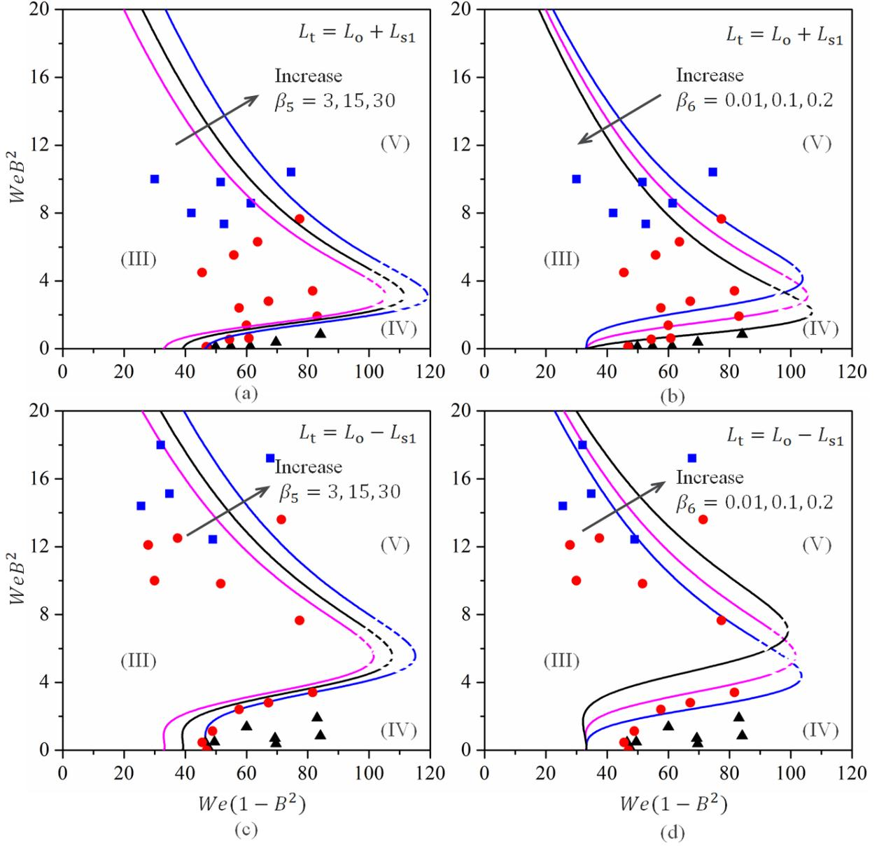
FIG. 14. Comparison of the predicted boundary for separations upon the collision between a spinning and a non-spinning droplet in Fig. 9. For sensitivity analysis, different values of  $\beta_5$  and  $\beta_6$  in large ranges are shown as (a)  $\beta_5$  and (b)  $\beta_6$  for  $L_t = L_o + L_{s1}$ ; (c)  $\beta_5$  and (d)  $\beta_6$  for  $L_t = L_o - L_{s1}$ .
