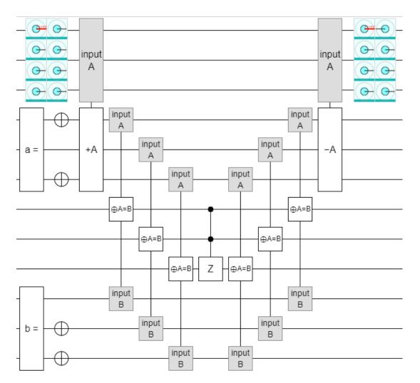
Fig. 13. 3-qubit Oracle function for solving the example equation
