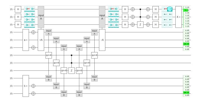
Fig. 14. 3-qubit Grover's Search Algorithm solving the simple equation with result X = 001
