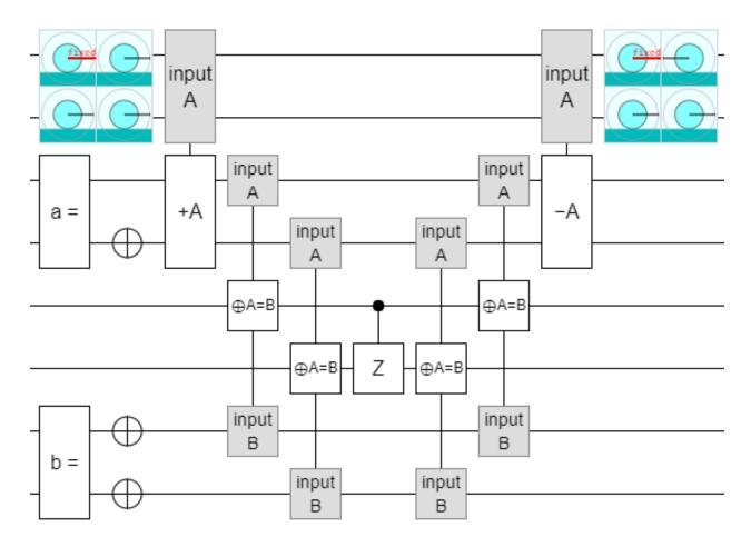
Fig. 11. Oracle function for solving the example equation
