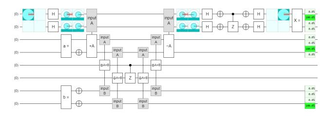
Fig. 12. Grover's Search Algorithm solving the simple equation with result X = 01
