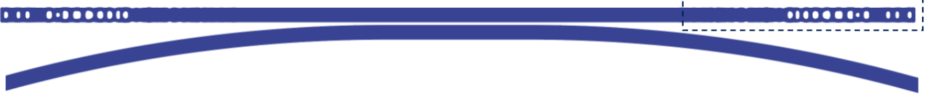
FIG. S3. Schematic of side coupled inverse designed FP resonator with selective reflection bands. This FP is coupled through a directional coupler due to the flexibility in tuning of coupling strength by tuning the gap size instead of targeting a particular through coupling strength. The gap size is chosen to be 100 \text{ nm} .
