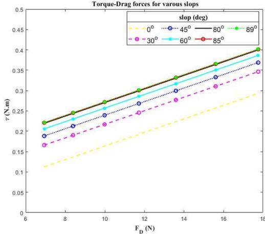
Fig. 6. Investigating the simultaneous effect of drag force change due to robot speed change and pipe slope on motor torques
