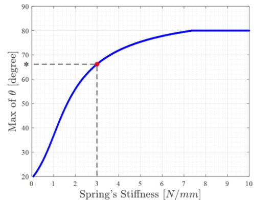
Fig. 4. Maximum allowable value for  $\theta$  angle in each spring's stiffness. To have a contact between the upper arm and the pipe,  $F'_N$  has to be positive. By substituting different values for  $k$  in (4), we can find permissible range for  $\theta$  that results in positive values for  $F'_N$ .
