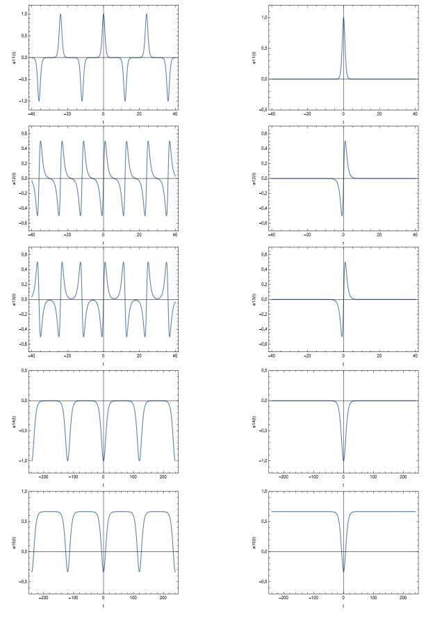
FIG. 5. Wave profiles of the five bound states  $a_{1j}$  (j = 1, 2, 3, 4, 5) given by eqs. (13)-(16), for k = 0.98 (left column) and k = 1(right column).
