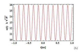
FIG. 1. Elliptic-soliton solution to the nonlinear amplitude equation (2), for two different values of the parameter of pulse dispersion k: (a) Periodic network of sharp pulse signals for large dispersion parameter (k = 0.98), (b) Elliptic-wave decay into a quasi-continuous signal for small dispersion parameter (k = 0.6).
