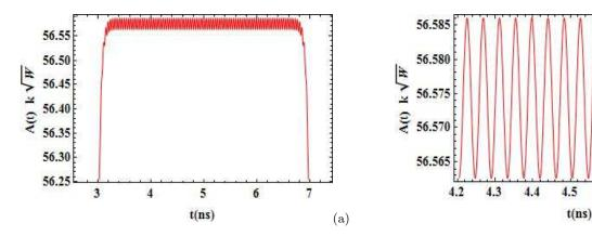
FIG. 3. Numerically reconstructed signal at the pumping rate  $\tau_A = 23.248 \text{ 1/ns}$ : (a) Double time scale comb-like pulse, (b) Apex of the large pulse: Soliton crystal of finite length.
