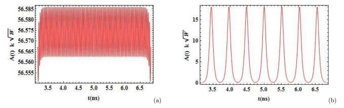
FIG. 4. Autocorrelation trace of the reconstructed signal: (a) Strong modulation illustrated by the amplitude gap between the soliton crystal and the large pulse, (b) Minimal modulation at the threshold frequency.
