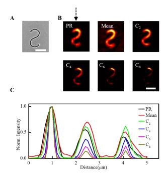
Fig. S2. Super-resolution imaging for a nanoscale object. (A) The SEM image of nanoscale object (~  $4 \mu m x 2 \mu m$  with line width of 200 nm). (B) Reconstruction images. (C) The intensity profile along the line indicated by the dashed arrow in (B). Scale bar: 2.5  $\mu m$ .
