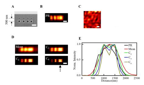
Fig. 5. NISSFI with artificial fluctuating emitters. (A) The artificial object created by vertically shifting the 4-dot sample by 500 nm. (B) PR result from the averaging speckle frame. (C) Estimated PSF. (D) Reconstructed images by NISSFI at different cumulant orders. (E) The intensity profile along the line indicated by dashed arrow in (D). Scale bar:  $1.0 \,\mu\text{m}$ .
