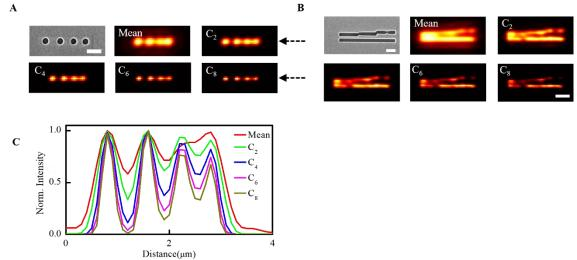
**Fig. S1. Experiment results of conventional SOFI without scattering media.** (**A**) SEM image and reconstruction images of the dot object at different cumulant orders. (**B**) SEM image and reconstruction images of separated lines with different gaps. (**C**) The cross-section indicated by dashed arrow in (**A**). Scale bar: 1.0 μm.
