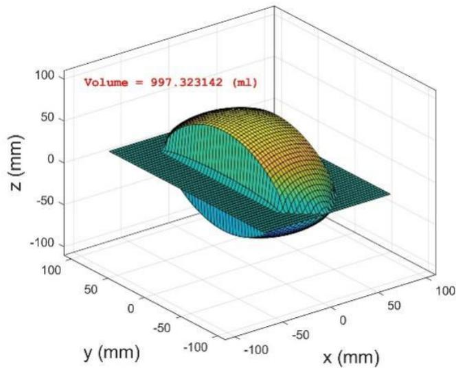
**Figure 6. Simulation of AMBU bag at  $d = 30mm$ .**
