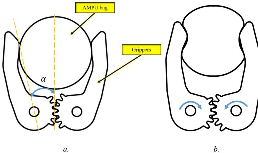
**Figure 3. Determination between grippers and AMBU bag.**
