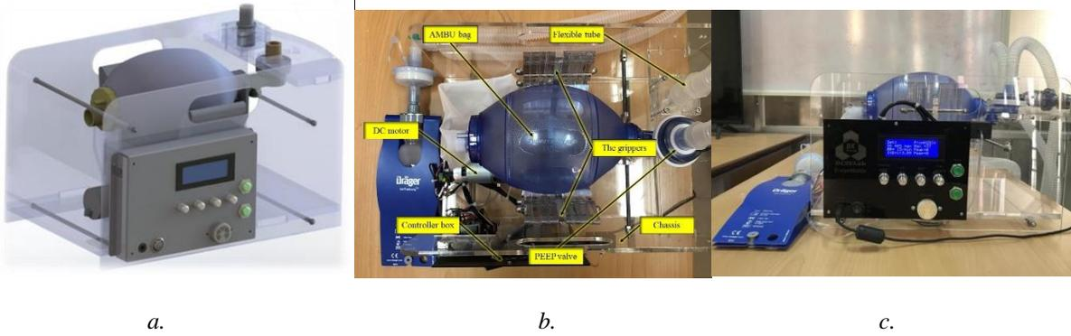
**Figure 2. The modeling to show the relationship between the grippers and AMBU bag.**
