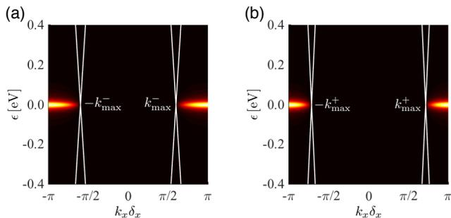
FIG. 10. Edge spectral functions of a bent graphene nanoribbon of width  $W = 192 \text{ nm}$  and bend curvature  $\lambda = 0.642 \mu\text{m}^{-1}$ . (a) The edge states on the stretched zigzag edge emerge from the Dirac points of the inner projected Dirac cones (white curves) at  $\pm k_{\text{max}}^-$ . (b) The edge states on the compressed zigzag edge emerge from the Dirac points of the outer projected Dirac cones (white curves) at  $\pm k_{\text{max}}^+$ .
