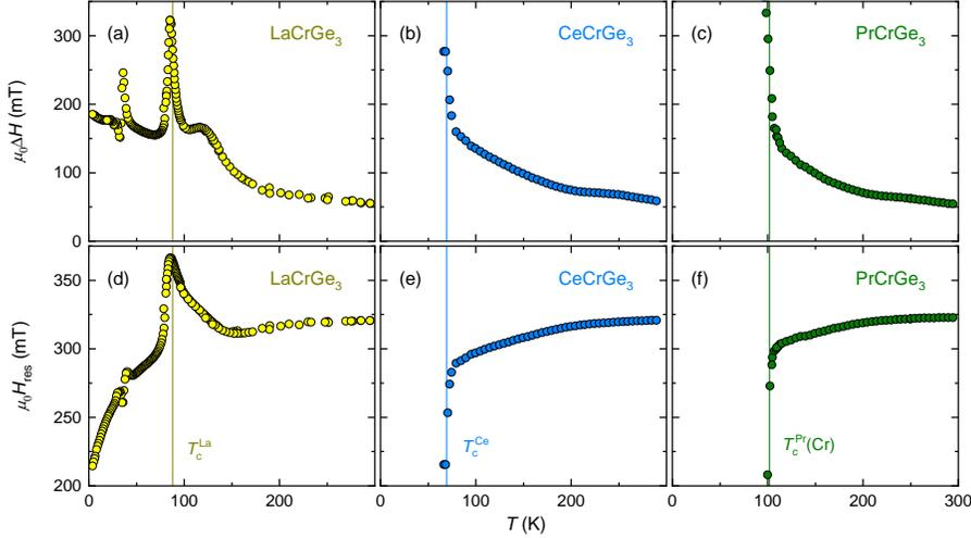
**Figure 5.** Linewidth  $\mu_0\Delta H$  and resonance field  $\mu_0H_{\text{res}}$ .  $T_C$  indicates the ferromagnetic ordering temperature.  $T_C$  was determined by the point of inflection in the  $\chi(T)$  data.
