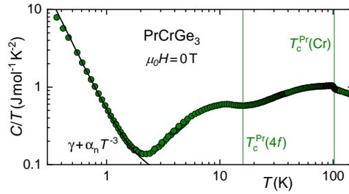
**Figure 2.** Temperature dependence of  $C/T$  of  $PrCrGe_3$ . At  $T < 2$  K the main contribution is the high temperature tail of the nuclear Schottky peak. The solid line is a fit with  $C_n/T = \gamma + \alpha_n T^{-3}$ .
