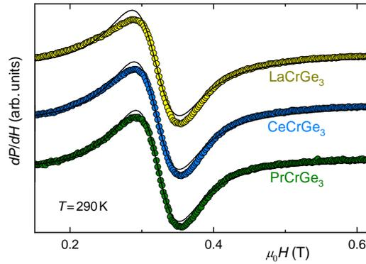
**Figure 3.** ESR spectra (symbols) at  $T = 290\text{ K}$  for  $\text{LaCrGe}_3$ ,  $\text{CeCrGe}_3$ , and  $\text{PrCrGe}_3$  and Lorentzian shape (lines) with  $g = 2.10 \pm 0.02$  and  $\mu_0 \Delta H = 55 \pm 2\text{ mT}$ .
