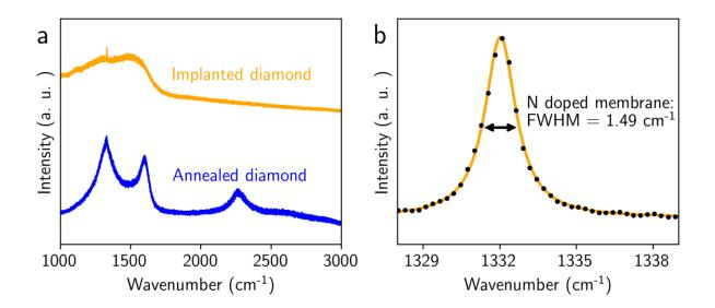
**Figure S2**: Additional Raman spectroscopy for membrane formation and overgrowth. (a) Orange curve: the implanted diamond substrate prior to annealing. Blue curve: the annealed diamond substrate. (b) The Raman peak for an isotopically purified,  $\approx 250$  nm overgrown membrane at 700 °C (40 h growth, back-etched down to 110 nm). The peak is at 1332.03(30) cm<sup>-1</sup>, with linewidth 1.486(14) cm<sup>-1</sup>.
