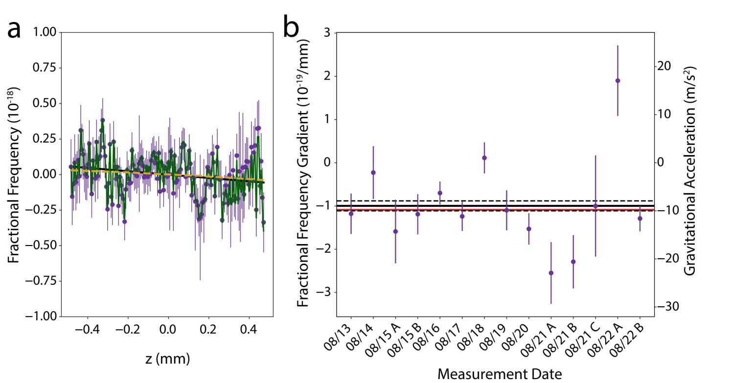
**Figure 4:** *In-situ* synchronous clock comparison. **a**, The cloud is separated as in Fig. 2a. The gravitational redshift leads to the higher clock(blue) ticking faster than the lower one(red). The length scale is in millimeters. **b**, Allan deviation of the frequency difference between the two regions in **a** over 92 hours. Purple points show differential stability fit by the green line. The single atomic region instability is shown in gold.
