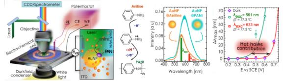
**Figure 19.** Plasmon-mediated polyaniline, PANI, electrodeposition on single Au NP triggered by laser LSPR excitation and probed by hyperspectral DFM. Adapted with permission from [227].
