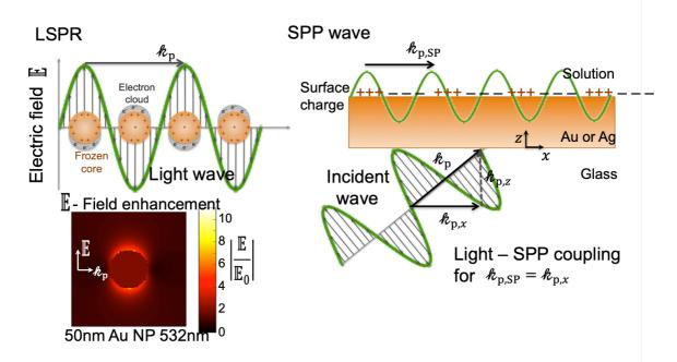
**Figure 3.** Generation of surface plasmons. (Left) Localized surface plasmon from the interaction of the electric field  $\mathbb{E}$  of light with the free electrons of an atom/spherical NP (Drude model) and associated  $\mathbb{E}$ -field enhancement in the near-field of a 50nm Au NP illuminated by a 532nm light (with propagation and  $\mathbb{E}$  directions). (Right) Conditions for producing propagating surface plasmon at surfaces (*e.g.* SPR microscopy).
