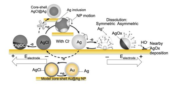
**Figure 22.** Examples of NP intermediates and mechanistic insights probed by optical microscopies during nanosilver electrochemistry.
