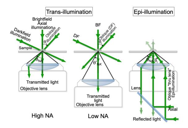
**Figure 9.** The numerical aperture, collection angle and mode of illumination/collection with a microscope objective.
