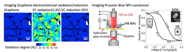
**Figure 21.** Left: IRM visualization of the reversible oxidation $\leftrightarrow$ reduction of Graphene $\leftrightarrow$ GO; adapted from [244] with permission. Right: Bright field transmittance imaging of single PB $\leftrightarrow$ PW nanocube electrochemical conversion. From [246] with permission.
