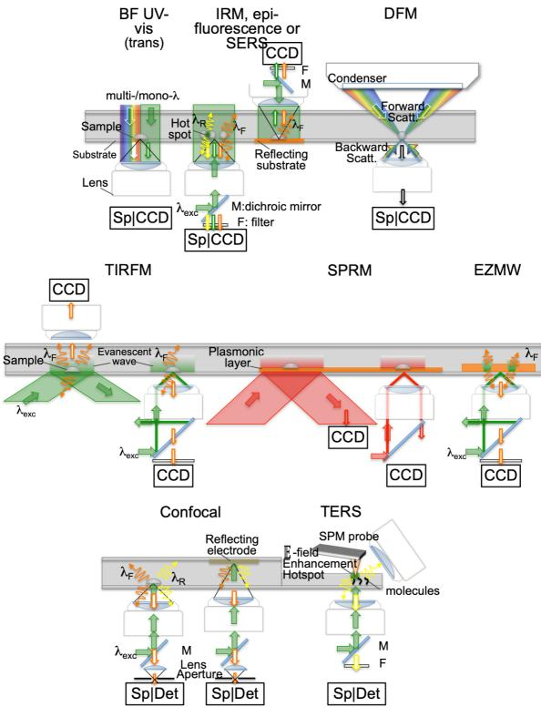
**Figure 8.** Illustration of configurations of optical microscopies to image the electrochemistry of a sample with an objective lens equipped with different detectors such as spectrograph (Sp) and a CCD camera or photomultiplier tube, PMT, detector (Det).
