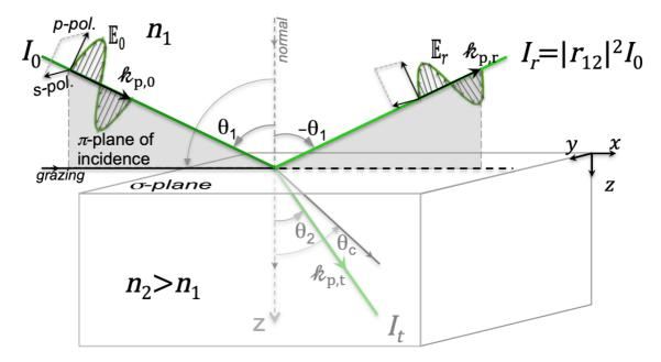
**Figure 2.** Reflection and transmission of an incident light beam of electric field  $\mathbb{E}_0$  propagating in an optical medium ( $n_1$ ) and impinging with oblique incidence (angle  $\theta_1$  to normal) the interface with a different optical medium ( $n_2$ ).
