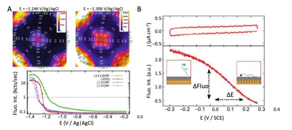
**Figure 17.** Fluorescence imaging of the electrochemistry of SAMs on Au electrodes. (A) Facet-dependence of SAMs electrodesorption illustrated from overlay of fluorescence images and electrode crystalline orientation map and fluoro-voltammograms. From [192] with permission. (B) Similarly the potential-induced orientation of diluted DNA in SAMs is probed from the fluoro-voltammogram, from [195] with permission.
