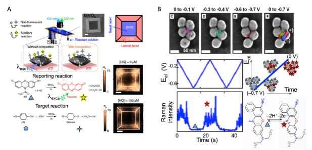
**Figure 18.** Super-localized adsorbates electrochemistry using (A) fluorescence or (B) SERS microscopies. (A) Strategy for evaluating the photooxidation of non-fluorescent probe (HQ) using a competition reaction. Adapted with permission from [208]. (B) Correlated SEM/SERS images of the potential dependent localization of Nile blue electron transfer on Ag NPs aggregates. Adapted with permission from [213].
