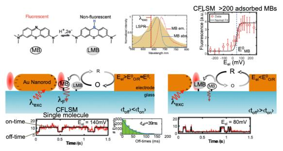
**Figure 11.** Confocal fluorescence microscopy of the redox switching at few to single adsorbed MB molecules. Fluorescence is enhanced by near-nanorod  $\mathcal{E}$ -field-enhancement. At the single MB level,  $E^{0}_{MB}$  is obtained from  $\langle t_{on} \rangle / \langle t_{off} \rangle$ . Adapted with permission from [141].
