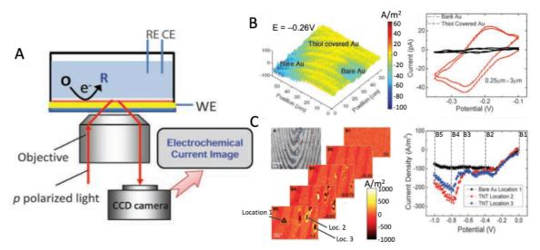
**Figure 16.** Quantitative SPRM imaging of the electrochemistry of molecular adsorbates on Au electrode. (A) Principle. (B) Imaging the heterogeneity of a thiol SAM from local SPRM-inferred voltammogram of a redox probe. (C) Imaging the electrochemical activity of fingerprint-coated electrode, showing local electron transfer blocking of fingerprint-coated regions and local reduction of TNT adsorbates (locations 2&3). From [100] with permission.
