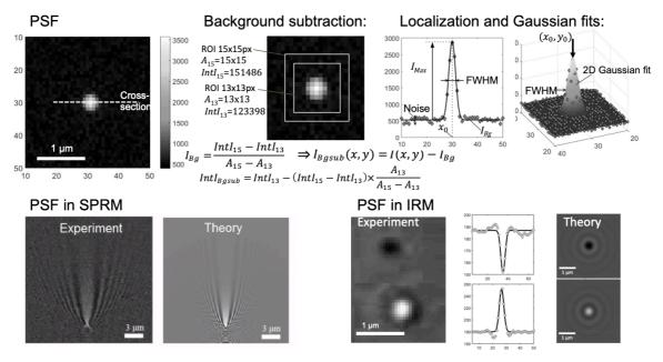
**Figure 10.** (Top) Extracting quantitative information from optical images: background, noise, localization, 1D or 2D PSFs. (Bottom) Interference-like PSF: large parabolic or ring-disks are predicted and observed in SPRM (adapted with permission from [96]) or IRM respectively; a Gaussian fit applies for the latter.
