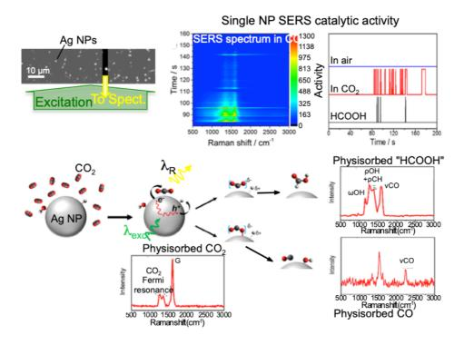
**Figure 13.** Principle of SERS imaging of  $CO_2$  photocatalysis through  $CO_2$  or reduced intermediates physisorption events at single Ag NP aggregates. Adapted with permission from [176].
