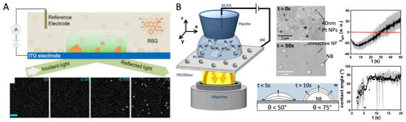
**Figure 15.** Imaging the formation of  $H_2$  gas NBs (A) at ITO by single molecule TIRFM and (B) at single Pt NPs by IRM. (A) Principle and evolution of the number of NBs detected with the electrode potential; from [86], with permission. (B) The quantitative NB growth deduced from  $I_{opt}$  variations allows estimating the dynamic evolution of the NB contact angle,  $\Theta$ , from [185].
