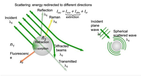
**Figure 5.** Schematic geometric-optics ray-approach of the different sources of interaction of light with a sphere: transmission and extinction by scattering and absorption with possible emission (fluorescence) or inelastic scattering (Raman). From the interaction of the incident plane wave with the sphere (see Figure 3), a resulting spherical scattered wave is produced.
