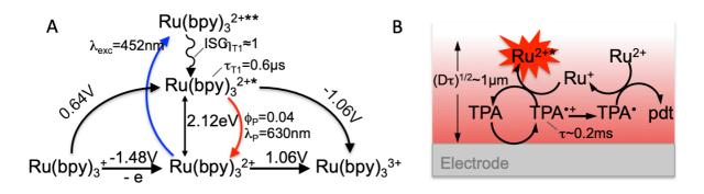
**Figure 7.** Principle of ECL. (A) energetics of the  $Ru(bpy)_3^{2^+}$  luminophore, and (B) chemicallylimited lighting of thin layer of solution exploiting the limited lifetime of the electrogenerated intermediate radicals of a coreactant.
