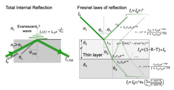
**Figure 4.** Schematic description of TIR illumination of an interface between two media  $(n_2, n_1)$ , and of the Fresnel formalism at a two-interfaces between three media with reflection/absorption/transmission of a light beam, e.g. at a sample  $(\widetilde{n_2})$  intercalated between an electrode  $(\widetilde{n_3})$  and electrolyte  $(n_1)$ .
