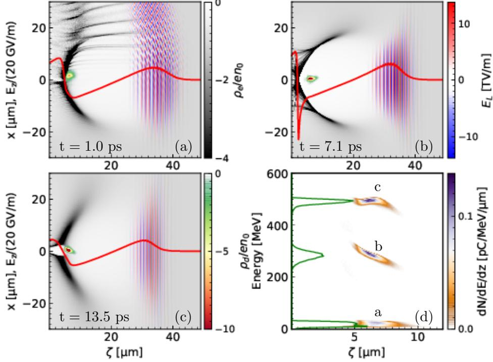
FIG. 6. Plots of a 3D PIC simulation. The driver pulse has  $a_0 = 2.74$ , the trigger pulse has  $a_1 = 1.37$ , and the collision angle is  $\theta = 8^\circ$ . The snapshots are taken (a) short after colliding, (b) at about 2 mm acceleration distance and (c) at about 4 mm acceleration distance. (d) The phase space distribution and energy spectrum (green curves) of the trapped electron beam at the time corresponding to the above three snapshots.
