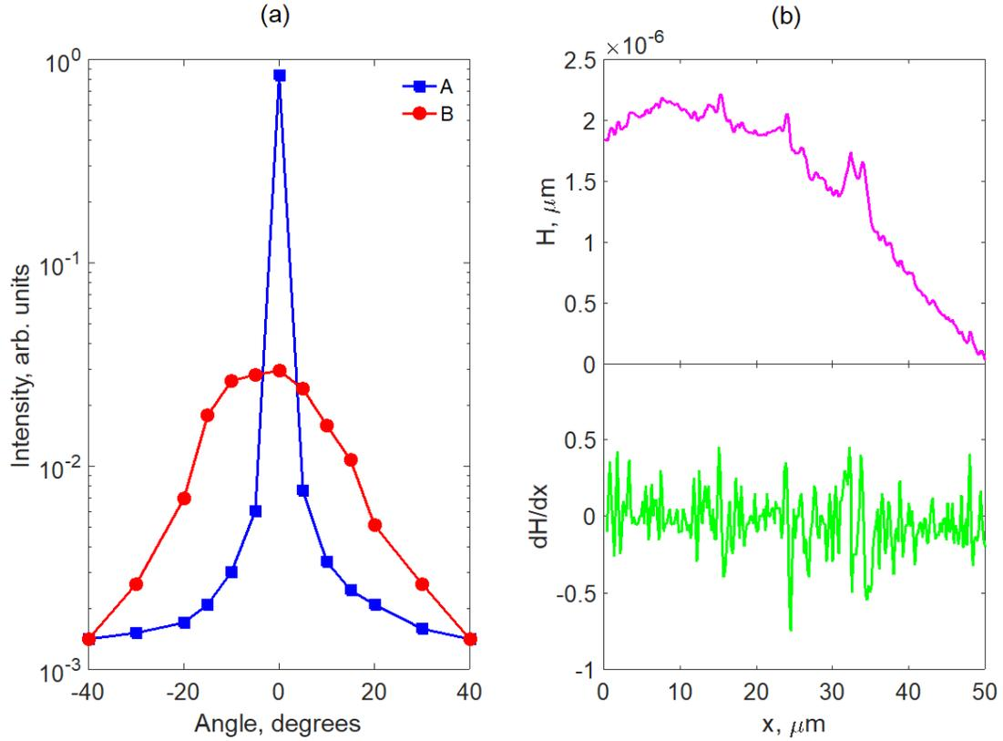
Fig. 6. Experimental specimen containing diffuse aluminum WF. (a) The intensity of scattered light in a certain direction as a function of the angle between this direction and the optical axis. Curve A relates to the parts of the specimen with the upper polymer slab and curve B relates to the parts of the specimen without the upper slab. (b) Relief cut (upper graph) and its first derivative (lower graph) measured by an atomic force microscope.
