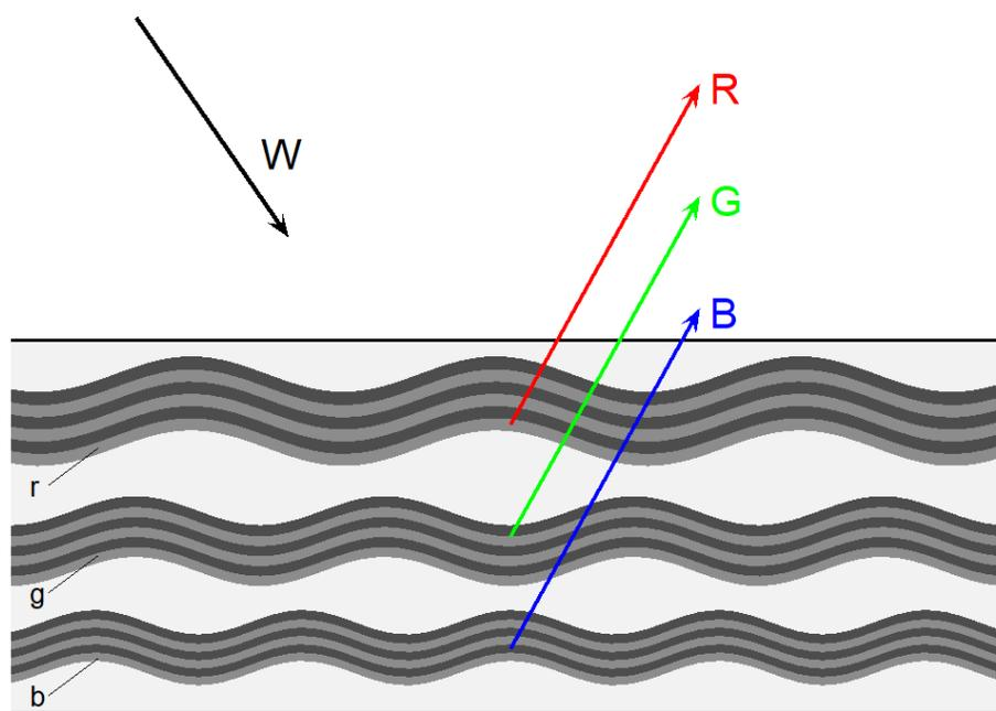
Fig. 2. Scheme of the proposed color hologram.
