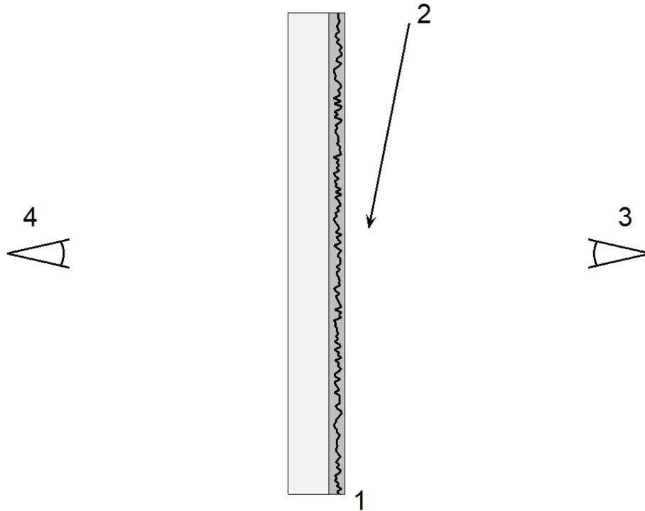
Fig. 5. Privacy window. 1 – OE with diffuse WF, 2 – back-light, 3 – outside observer, 4 – inside observer.
