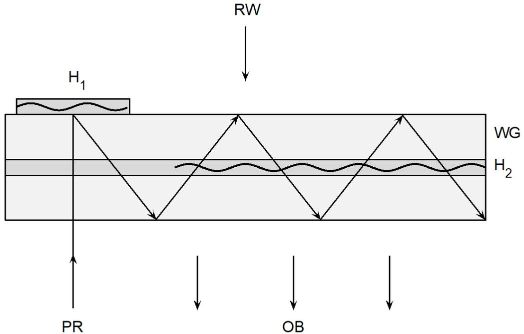
Fig. 7. Waveguide display. WG – waveguide, H1 – input hologram, H2 – output hologram, PR – beam from projector, RW – real world, OB – observer.
