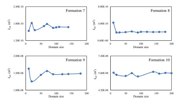
Fig. 1A. Plots of effective permeability against domain size to determine the representative elementary volume (REV) for each of the 2D formations.
