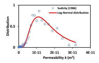
Fig. 1. The log-normal distribution, Eq. (8), with  $k_g = 1.5 \times 10^{-11} \text{ m}^2$ ,  $\sigma = 0.56$ ,  $k_{\min} = 6.1 \times 10^{-14} \text{ m}^2$ , and  $k_{\max} = 3.2 \times 10^{-11} \text{ m}^2$  fitted with  $R^2 = 0.80$  to the permeability histogram. Permeability measurements are from the Borden site (Sudicky, 1986).
