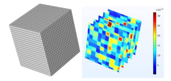
Fig. 2. (left) A 3D domain of size of 10 m with 20 cells along each side (domain size = 20), and (right) random spatial distribution of permeability values in the same domain.
