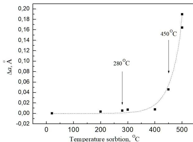
Fig. 1. The dependence of the lattice parameter  $a$  of the studied samples of  $C_{60}$  on the temperature  $T_s$  of saturation with gaseous  $N_2$  at a pressure of 30 atm on the base of experimentally obtained data [17].
