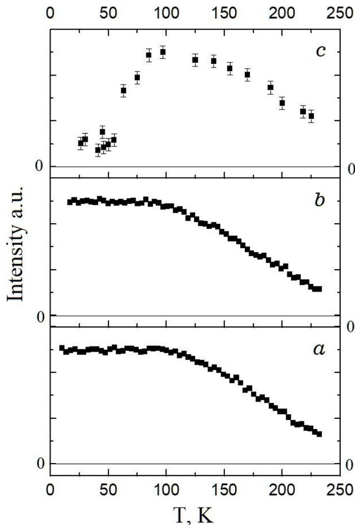
Fig. 2. Temperature dependences of the integrated radiation intensities of the  $C_{60}$  fullerite, normalized to the corresponding values at  $T = 25 \text{ K}$ : (a) - pure; (b) - intercalated  $N_2$  at 280 °C and a pressure of 30 atm for 150 hours (physical sorption); (c) - intercalated  $N_2$  at 450 °C and a pressure of 30 atm for 200 hours (chemical sorption). All curves are measured in the warming mode.
