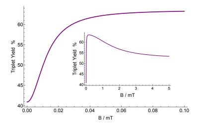
**Figure 2.** The dependence of the triplet yield of the [TrpH<sup>++</sup> ... O<sub>2</sub><sup>-</sup>] complex on applied static magnetic field for  $r = 10^5 \text{ s}^{-1}$ ,  $k = 10^6 \text{ s}^{-1}$ ,  $a_A = 1.6046 \text{ mT}$ . The triplet yield goes from around 60% to around 40% by changing the magnetic field strength from GMF to HMF. The strong HMF effect is further emphasized by the inset.
