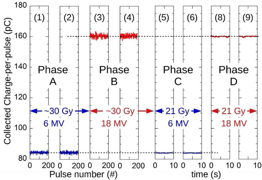
**Figure 5.** Collected charge-per-pulse values at 6 MV (red) and 18 MV (blue) X-rays recoded by the proposed prototype (1-4) and those estimated by measurements carried out by means of a Keithley 6517A electrometer (5-9) (see text). Odd and even numbers refer to the beginning and the end, respectively, of each phase (from A to D). The total detector's absorbed dose in each phase is also reported.
