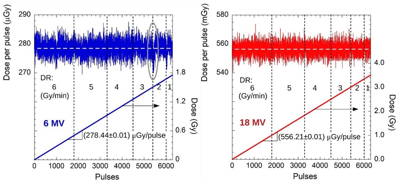
**Figure 7.** Dose per pulse and total collected dose recorded by the proposed prototypal system for different DRs. An average value of about 0.278 and 0.556 mGy/pulse, at 6 MV and 18 MV, respectively, is found, Cumulative sum of dose (continuous lines) displays a slope in excellent agreement to the expected DP value.
