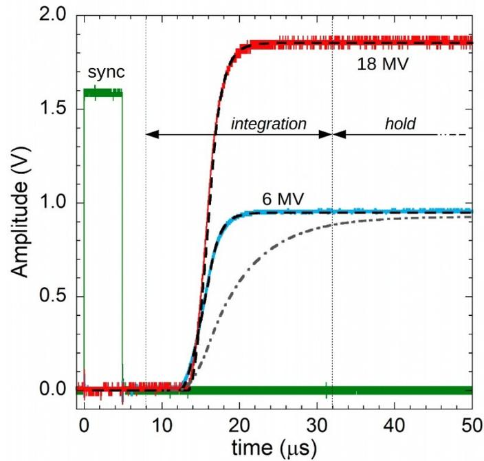
**Figure 2.** Typical output voltage  $V_o$  of the proposed readout electronics for 6 MV (blue) and 18 MV (red) X-ray pulses impinging on the CVD-diamond dosimeter. Sync signal (green) is used to synchronize the  $S1$  and  $S2$  control signals. Dotted lines represent simulations (see text).
