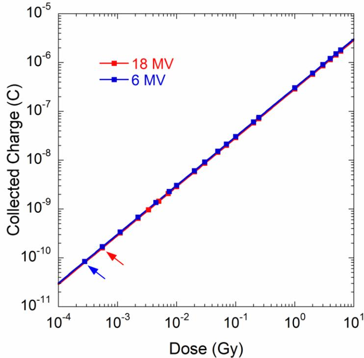
**Figure 6.** Collected charge as a function of dose for X-ray photons emitted at 6 MV and 18 MV. Data for dose lower than 1 Gy have been acquired by the proposed prototype, whereas a Keithley 6517A electrometer was used in the 1-6 Gy range.
