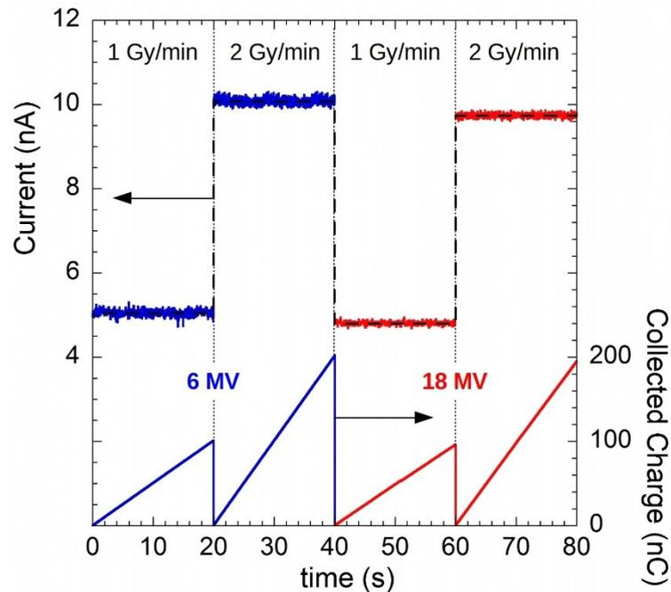
**Figure 4.** Detector photocurrent and collected charge at different dose rates for X-ray photons emitted at 6 MV and 18 MV as processed by the proposed detection system.
