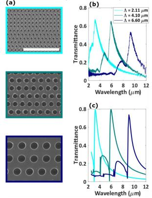
Figure 5. (a) SEM pictures of three laser-fabricated EOT metasurface devices with increasing geometrical periods (scalebar is 10  $\mu$ m). (b) FTIR measurements of the fabricated samples, revealing a progressive increase of the transmission peak wavelength as the period increases. The results are in very good agreement with the numerical simulations shown in (c).
