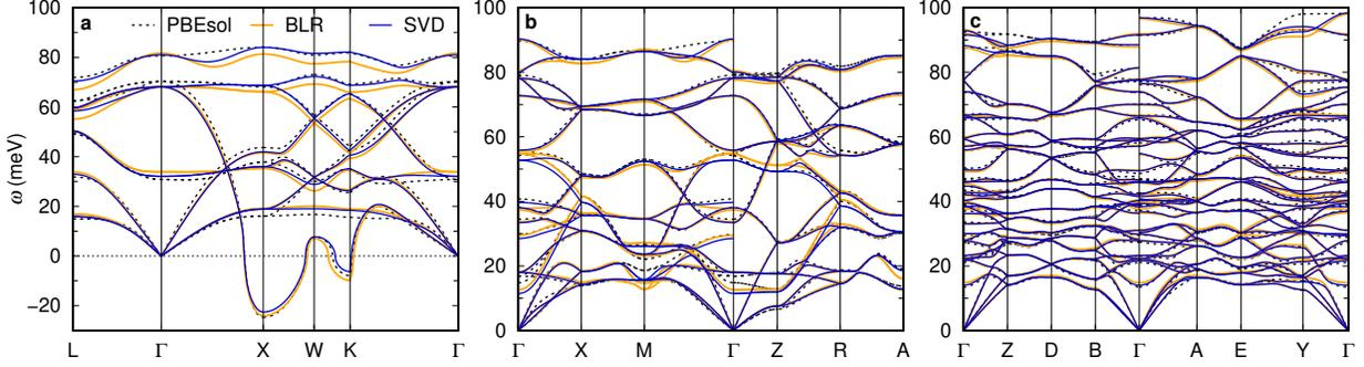
**Fig. 3. Prediction of phonon frequencies.** Phonon dispersions of **a** cubic, **b** tetragonal, and **c** monoclinic  $\text{ZrO}_2$  along high-symmetry lines in the Brillouin zone. The results obtained using the MLFFs trained with BLR (orange lines) and SVD (blue lines) for the regression are compared with the AI ones calculated using PBEsol (dashed black lines).
