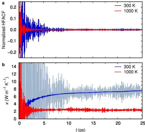
**Fig. 5. Calculating the thermal conductivity using GK theory. a** Heat-flux autocorrelation function (HFACF) normalized by its zero-time value and **b** thermal conductivity as a function of correlation time at  $T = 300$  K and 1000 K. In **b**, the moving average of  $\kappa$  over blocks of 1000 time steps is shown on top of the raw data at  $T = 300$  K.
