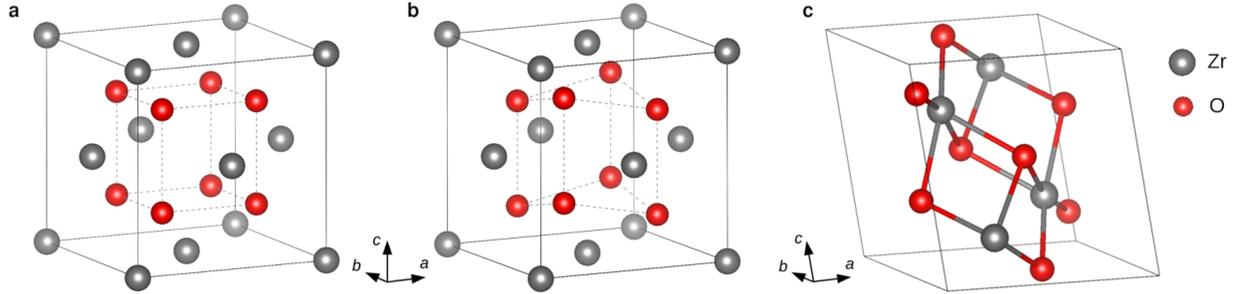
**Fig. 1. Crystal structures of zirconia.** Ball-and-stick model of the three structural phases of  $\text{ZrO}_2$ : **a** cubic, **b** tetragonal, and **c** monoclinic. The 12-atom conventional cells are represented, and the Zr-O bonds are shown only in the monoclinic structure.
