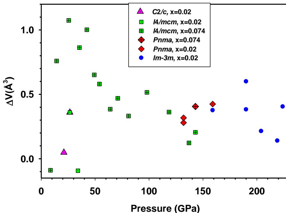
**Figure 9.** The pressure dependencies of the volume difference between the doped and undoped  $((\text{CH}_4)_x(\text{H}_2\text{S})_{(1-x)})_2\text{H}_2$  compounds in various phases and with various composition  $x$  investigated in this work.
