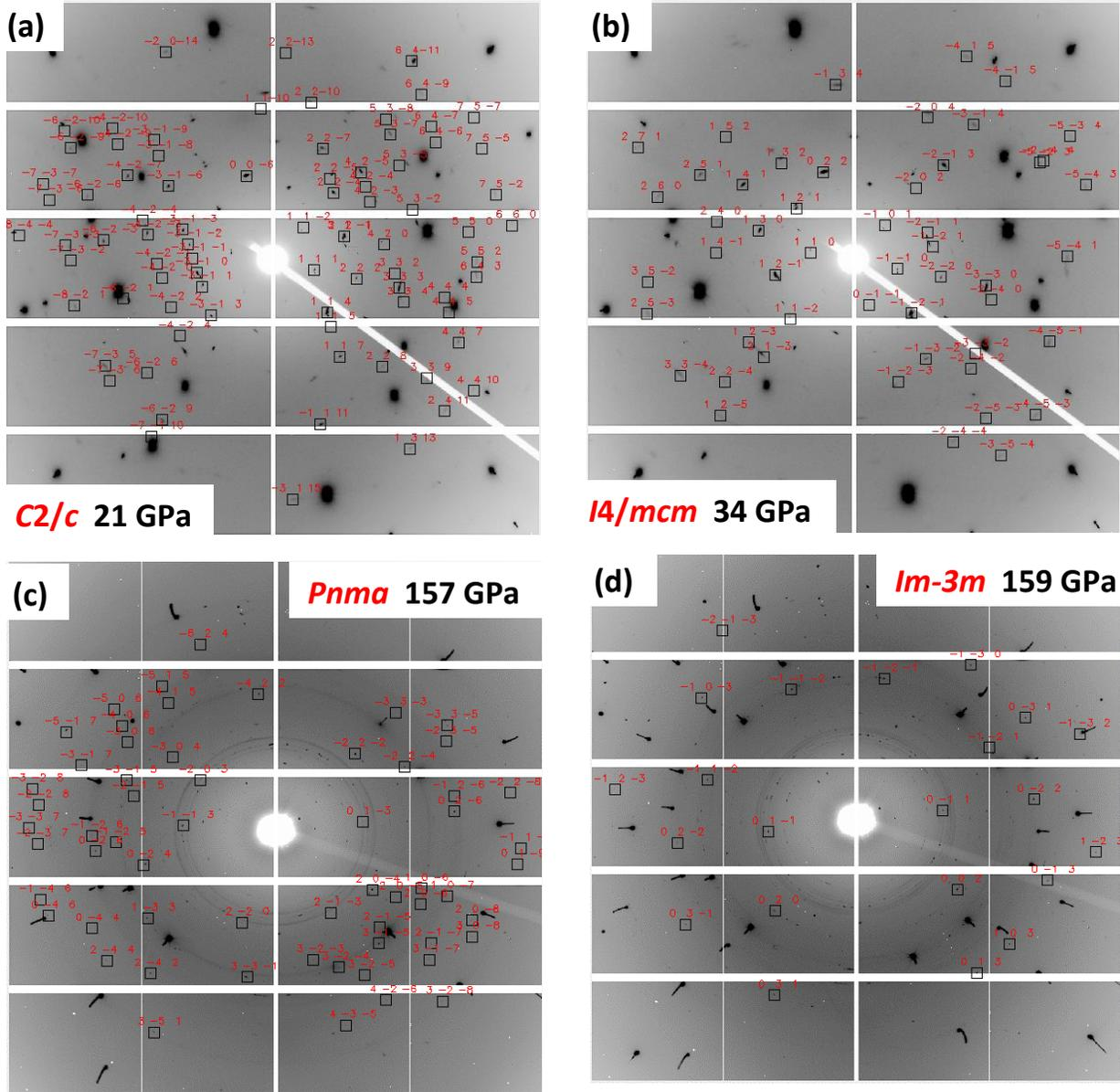
**Figure 5.** Single crystal XRD diffraction at high pressures of the documented phases of  $((\text{CH}_4)_x(\text{H}_2\text{S})_{(1-x)})_2\text{H}_2$  ( $x=0.02$ ). The patterns are taken in a wide scan mode in the range of the  $\omega$  rotations of  $\pm 10^\circ$  for  $C2/c$  (a),  $I4/mcm$  (b), and  $Pnma$  (c) phases and  $\pm 20^\circ$  for  $Im-3m$  (d) phase.
