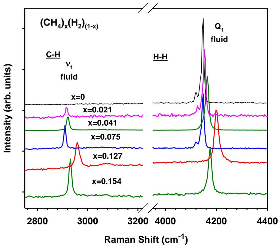
**Figure S1.** Raman spectra of the C-H and H-H stretch modes of  $(\text{CH}_4)_x(\text{H}_2)_{(1-x)}$  fluids after gas loading in the DAC, which served for determination of the  $\text{CH}_4$  content (Fig. 1(b)).
