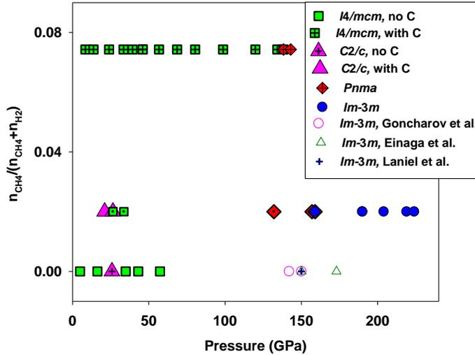
**Figure 7.** The pressure-composition phase diagram of ((CH<sub>4</sub>)<sub>x</sub>(H<sub>2</sub>S)<sub>(1-x)</sub>)<sub>2</sub>H<sub>2</sub> compounds. The structural data of this work are shown with filled symbols, while the stability of *Im-3m* H<sub>3</sub>S is indicated by open symbols following the results of Refs.<sup>9, 10, 30, 31</sup>. The *R3m* H<sub>3</sub>S detected at 70-140 GPa is not shown as it is likely metastable<sup>9</sup>.
