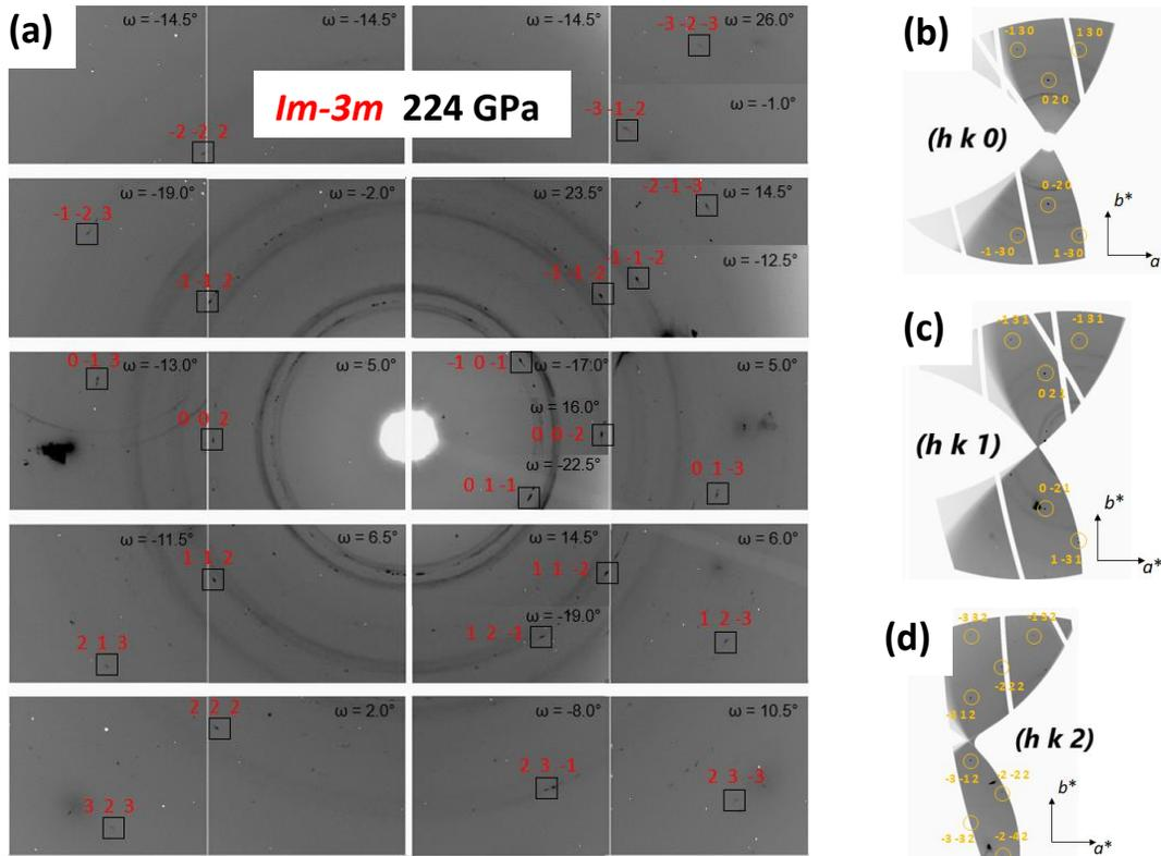
**Figure 6.** Single crystal XRD diffraction of  $Im\text{-}3m$   $((\text{CH}_4)_x(\text{H}_2\text{S})_{(1-x)}_2\text{H}_2$  ( $x=0.02$ ) at 224 GPa. Panel (a) is a mosaic of patterns taken at the different  $\omega$  rotations angles, demonstrating a variety of  $(hkl)$  reflections. The panels (b), (c), (d) show  $(hkl)$  slices of reciprocal space with attributed diffraction spots.
