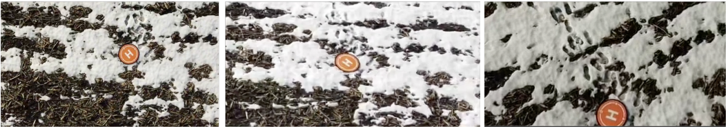
Fig. 6. Data Collection: (Left) UAV flying on top of the target object at high altitude (Middle) UAV flying at a distance from the target object, but its tilted camera angles capture the target object in the center of the screen (Right) UAV flying closer to the target object captures it at the bottom of the screen
