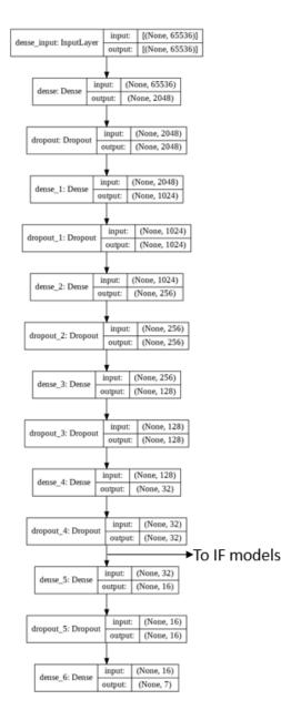
Fig. 1. Waveform classifier architecture with the output of the 32-node layer going to IF models
