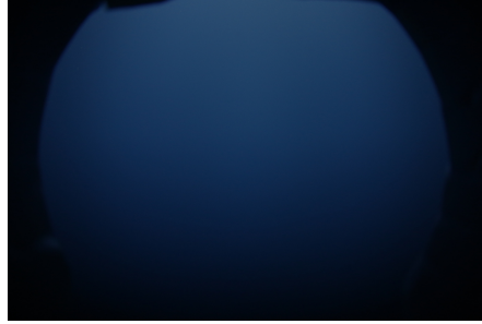
Figure 4: A water column image I_c(x, P_{\text{high altitude}}) taken by the AUV very high above the seafloor. It only shows scattering effects.
