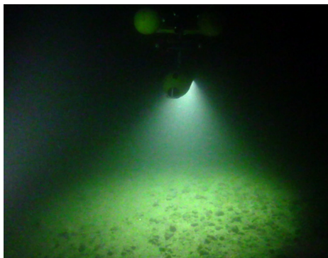
Figure 1: An autonomous underwater vehicle (AUV) in about 100m water depth photographing the seafloor. Multiple LEDs with angular fall-off create illumination cones towards the seafloor. The footprint of the superimposed cones depends on the AUV’s attitude and altitude, and the water body below the AUV scatters the light. Once the AUV moves on to the next photo, also the light will move on, making image matching and true surface color estimation very challenging.
