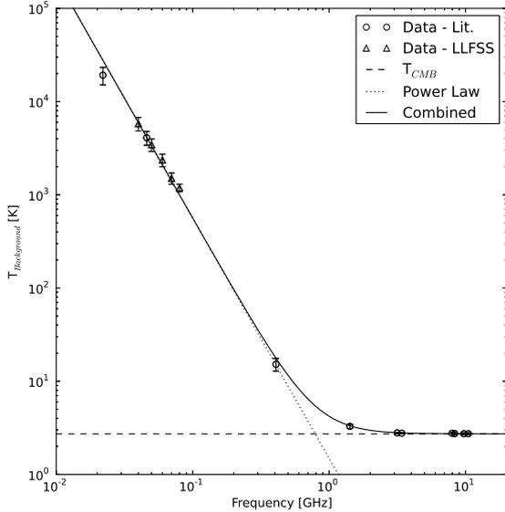
**Figure 1.** The measured radio background brightness spectrum in radiometric temperature units reproduced from [Dowell & Taylor \(2018\)](#), as measured by the few measurements and maps where an absolute zero-level calibration was either explicit or obtained, including that work. The brightness shows a clear power-law rise at frequencies below  $\sim 10$  GHz, above the otherwise dominant cosmic microwave background level represented by the dashed line.
